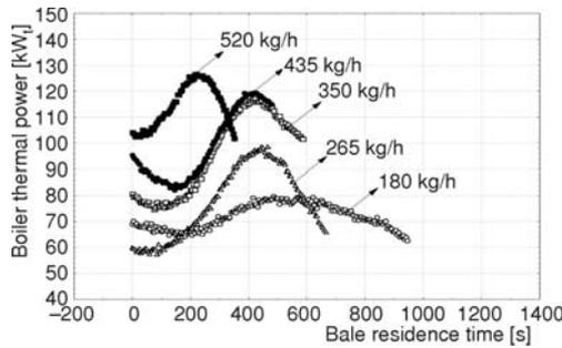
Figure 7. Correlation between boiler thermal power and bale residence time, experimental data, re-circulation 33%
