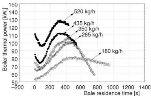
Figure 5. Correlation between boiler thermal power and bale residence time, experimental data, re-circulation 16.5%
