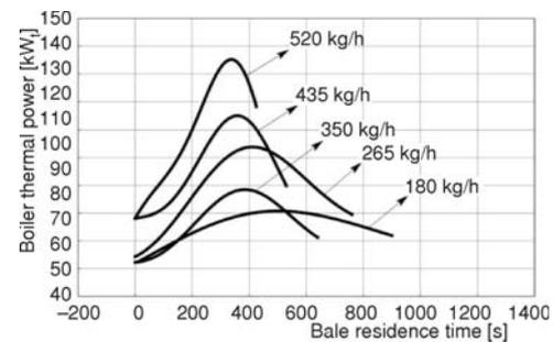
Figure 6. Correlation between boiler thermal power and bale residence time, model (1), re-circulation 16.5%
