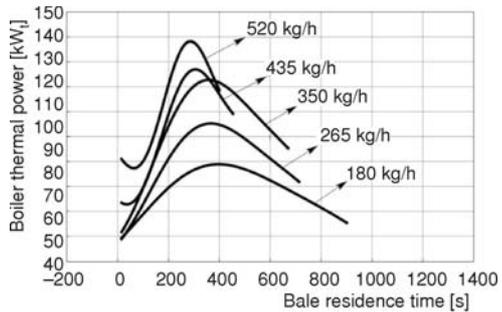
Figure 4. Correlation between boiler thermal power and bale residence time, model (1), re-circulation 0%
