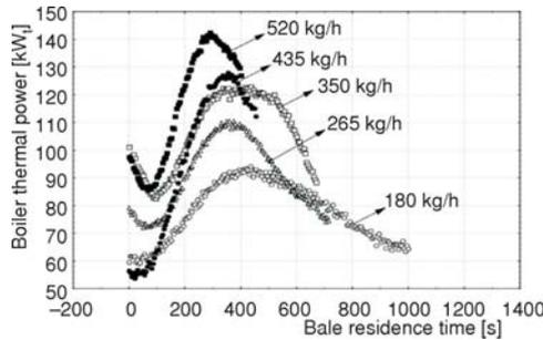
**Figure 3. Correlation between boiler thermal power and bale residence time, experimental data, re-circulation 0%**
