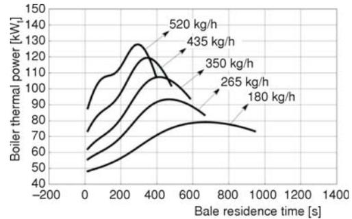
Figure 8. Correlation between boiler thermal power and bale residence time, model (1), re-circulation 33%
