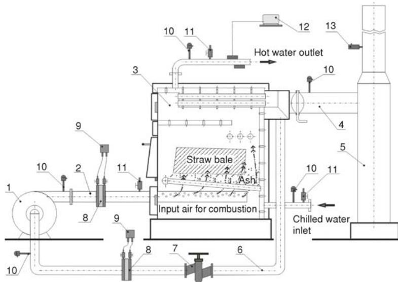
**Figure 1. Boiler plant of manufacturer “Ekoproduct” from Novi Sad with the measuring and regulation equipment**
