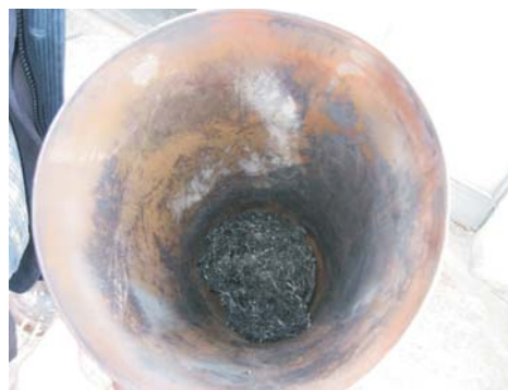
Figure 13. Photo of the ash on the grate, at the end of combustion process
