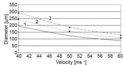
**Figure 1. Diameter of sprayed drops vs. their motion velocity (surface tension,  $\sigma$ : 1 – 0.040, 2 – 0.050, and 3 – 0.060  $\text{kg/s}^2$ )**
