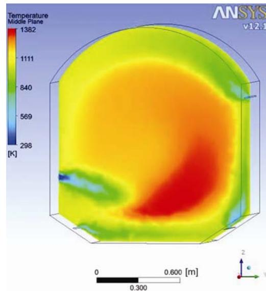
**Figure 7. Temperature field in the sprayer plane**
