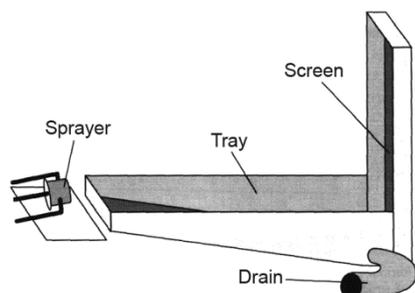
Figure 2. Test bench for WCF spraying tests
