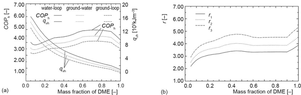
Figure 3. System performances vs. mass fraction of DME for water heater application
