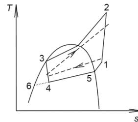
Figure 2. T-s diagram showing the CO<sub>2</sub>/DME based subcritical heat pump
