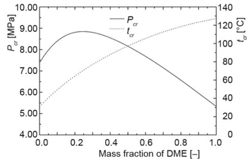
Figure 1. Critical pressure and temperature of CO<sub>2</sub>/DME mixture
