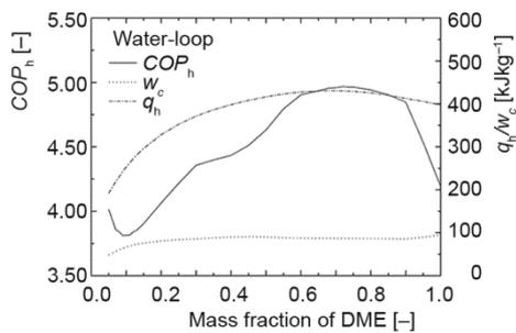
Figure 4. System performances vs. mass fraction of DME for water-loop water heater
