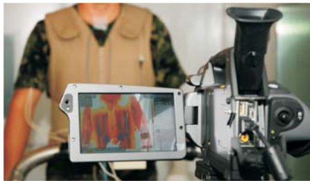
Figure 2. Application of IR thermography with camera FLIR SC620
