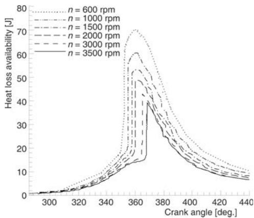
**Figure 6. Heat loss availability under various engine speeds**
