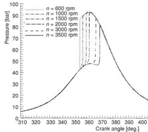
**Figure 2. In-cylinder pressure under various engine speeds**
