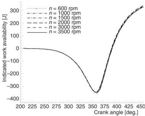
**Figure 5. Indicated work availability under various engine speeds**
