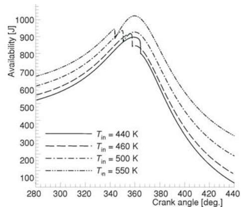
Figure 16. Total availability under various inlet charge temperatures
