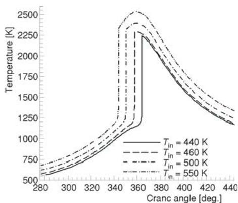
Figure 13. In-cylinder temperature under various inlet charge temperatures
