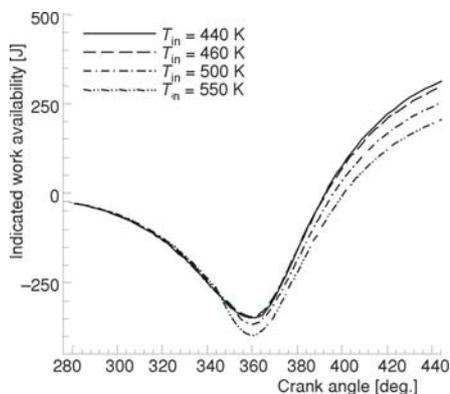
Figure 14. Indicated work availability under various inlet charge temperatures
