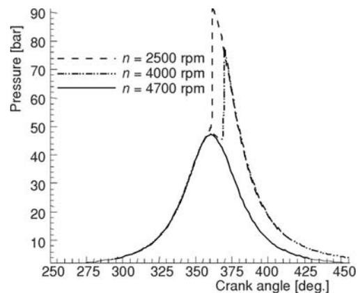
**Figure 4. In-cylinder pressure under various engine speeds**
