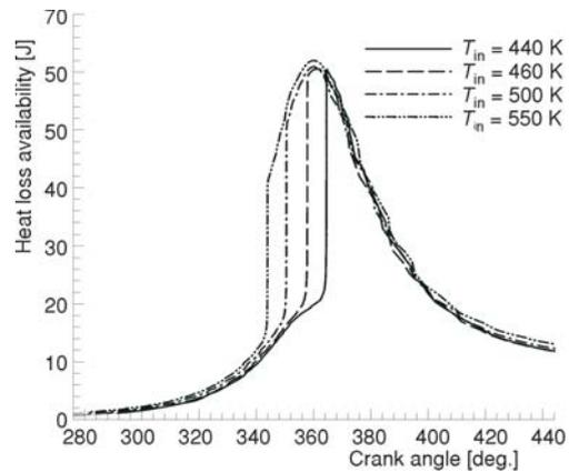
Figure 15. Heat loss availability under various inlet charge temperatures
