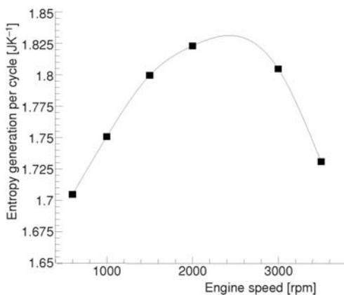
Figure 10. The effect of engine speed on entropy generation per cycle
