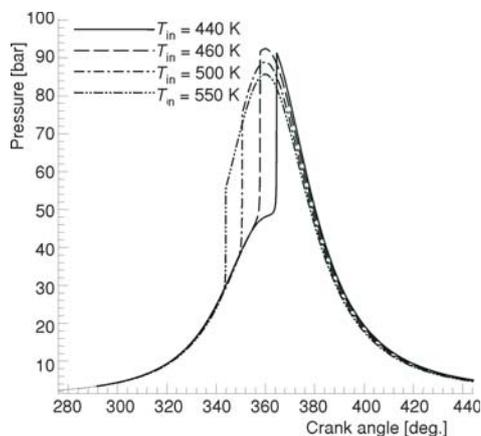
Figure 12. In-cylinder pressure under various inlet charge temperatures
