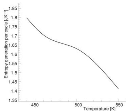
Figure 17. The effect of inlet charge temperature on entropy generation per cycle
