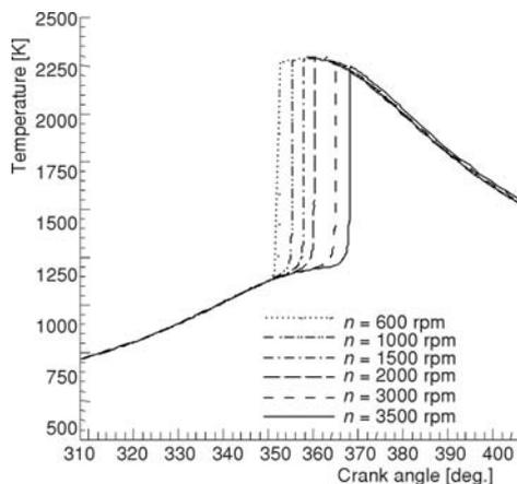
**Figure 3. In-cylinder temperature under various engine speeds**
