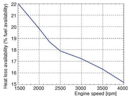
**Figure 8. The effect of engine speed on heat loss availability [12]**
