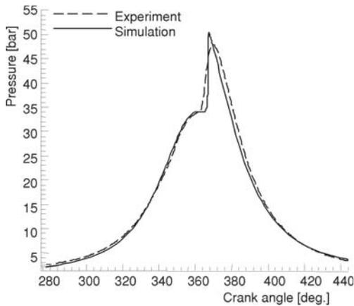
**Figure 1. Model validation under engine speed 600 rpm and inlet temperature 313 K**
