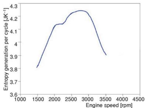
Figure 11. The effect of engine speed on entropy generation per cycle [12]
