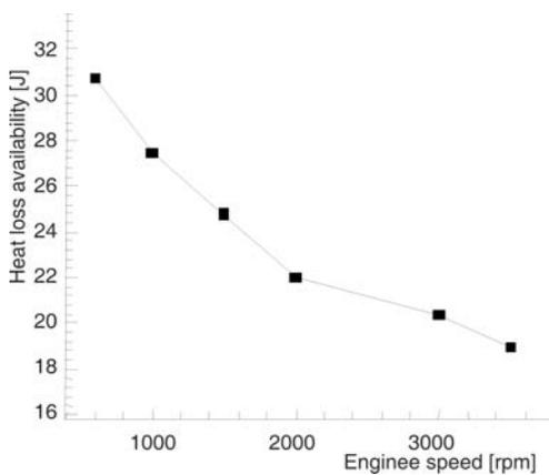
**Figure 7. The effect of engine speed on heat loss availability**
