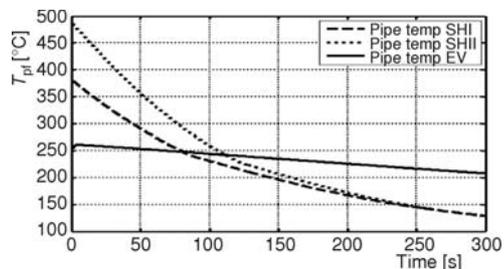
**Figure 5. Pipe temperature variation in superheaters 1 and 2 and evaporator during**
