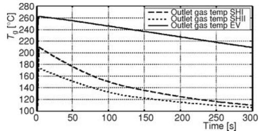
**Figure 3. Variation of outlet purge gas temperature from superheaters 1 and 2 and evaporator during purge time**
