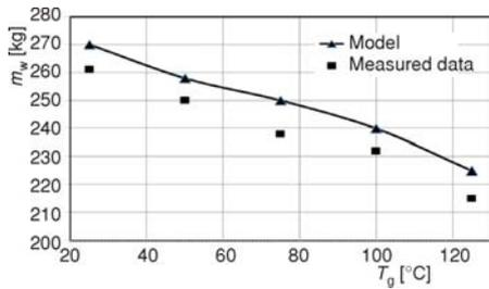
**Figure 7. Variation of condensate mass formation through purging time with purge gas temperature**
