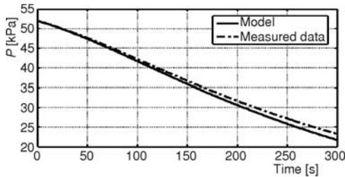
**Figure 2. Comparison of system pressure variation during purging time between model and measured data**
