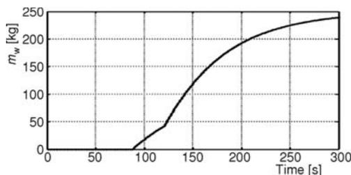
**Figure 6. Condensate mass formation during purge time**
