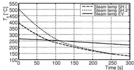
**Figure 4. Steam temperature variation in superheaters 1 and 2 and evaporator during**
