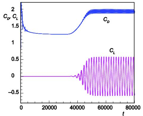
Figure 3. Drag coefficient and lift coefficient for the static elliptical cylinder by LB-DF/FD
