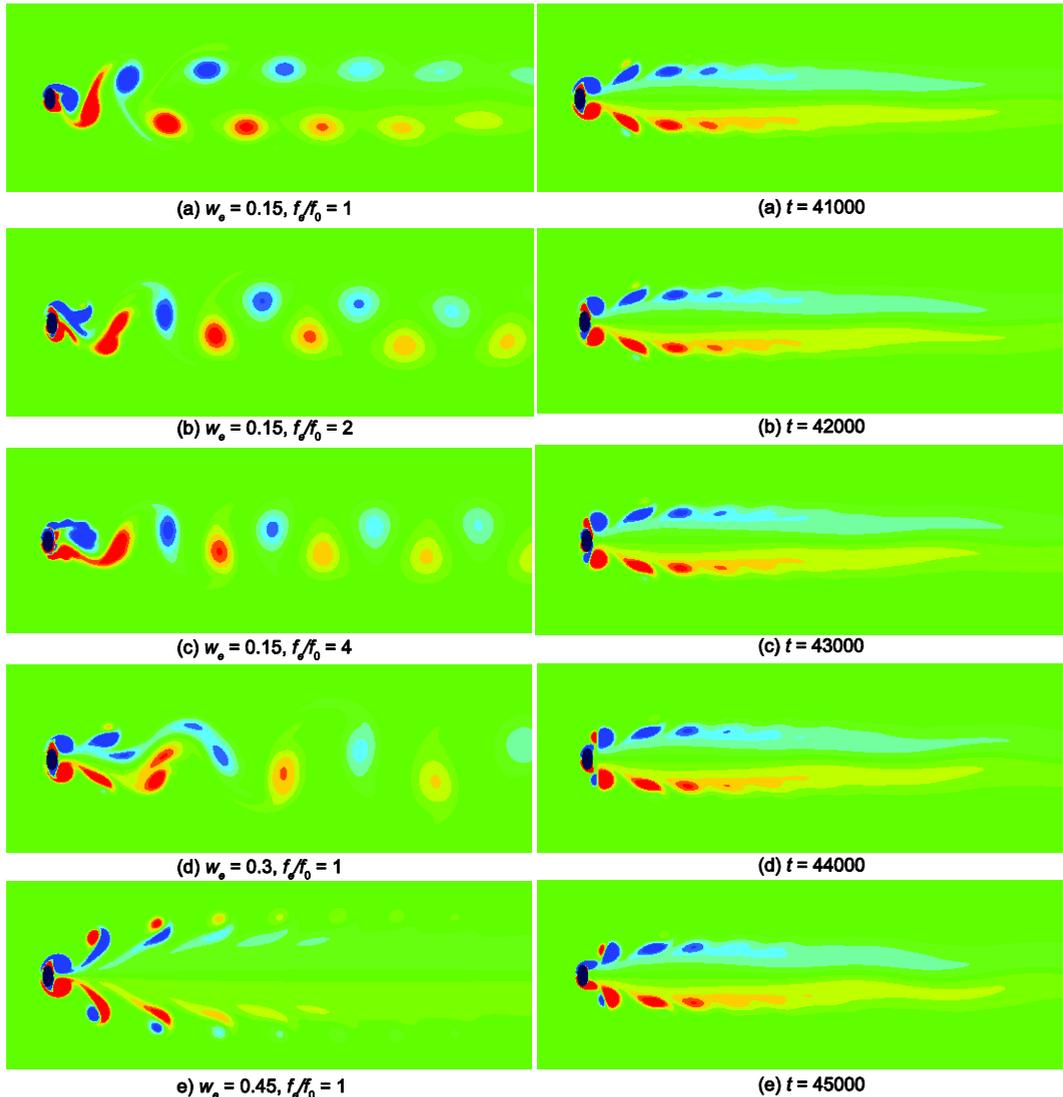
Figure 4. Vortex shedding patterns at different amplitude and frequency
