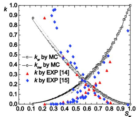
Figure 2. Relative permeabilities by Monte Carlo simulations and experimental data in Berea sandstone at porosity 0.240
