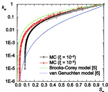
Figure 1. A comparison of the relative permeability for wetting phase between Monte Carlo simulations and empirical formulas
