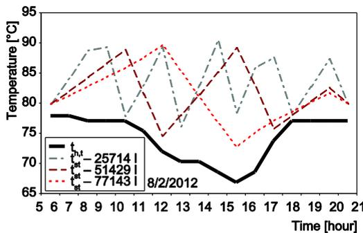
Figure 3. Profiles for water temperature in heat storage and supply water to consumers for 08/02/2012
