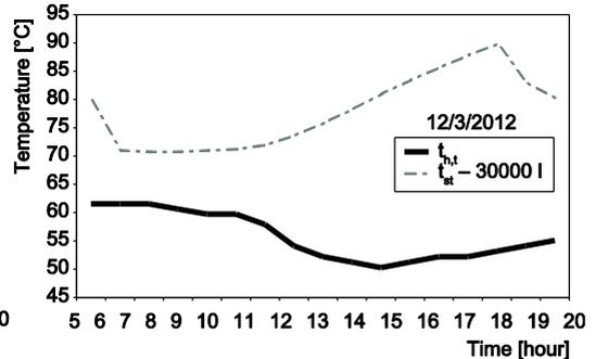
Figure 6. Profiles for water temperature in heat storage and supply water to consumers for 12/03/2012, working with two boilers
