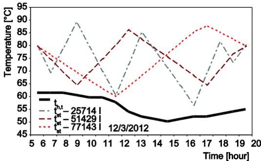
Figure 5. Profiles for water temperature in heat storage and supply water to consumers for 12/03/2012
