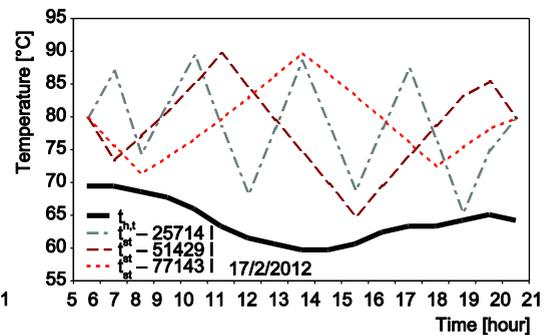
Figure 4. Profiles for water temperature in heat storage and supply water to consumers for 17/02/2012
