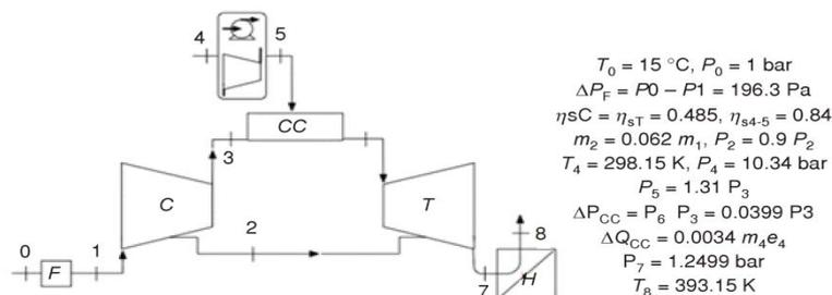
**Figure 1. Diagram and main cycle parameters of the standard gas turbine programmed with PATITUG**
