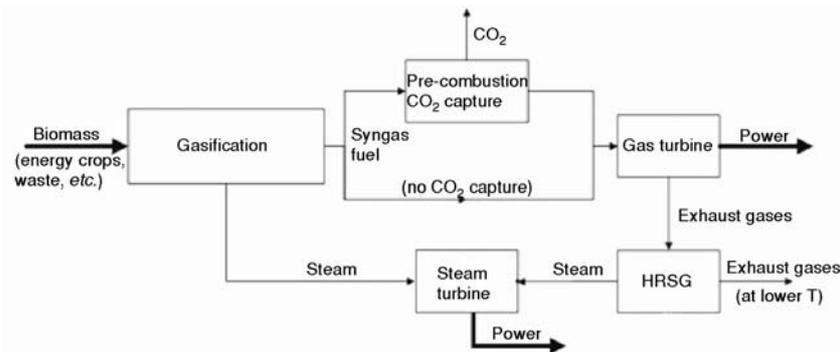
Figure 4. Block diagram of a BioIGCC power plant
