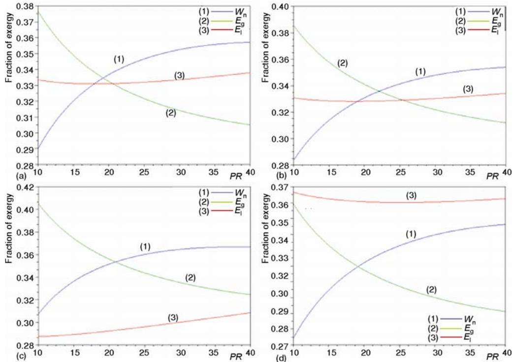
Figure 3. Exergy balances ( $TIT=1723.15$  K) for (a) pure methane, (b) biogas (53%  $CH_4$ , 42%  $CO_2$ , 4%  $N_2$ , 1%  $O_2$ ), (c) syngas (50%  $H_2$ , 50%  $CO$ ), and (d) pure ethanol, respectively. Values are expressed as fractions of the inlet exergy,  $m_4 e_4$
