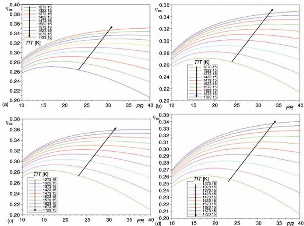
Figure 2. Brayton cycle exergetic efficiency as a function of  $PR$  (horizontal axis) and  $TIT$  (data series) for: (a) pure methane, (b) biogas (53%  $CH_4$ , 42%  $CO_2$ , 4%  $N_2$ , 1%  $O_2$ ), (c) syngas (50%  $H_2$ , 50%  $CO$ ) and (d) pure ethanol (color image see on our web site)
