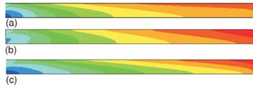
Figure 13. Contours of total temperature (a) k-\epsilon , (b) RNG, and (c) SST k-\omega
