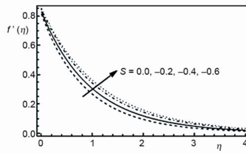
Figure 3. Velocity profiles for various values of  $S$  (blowing)
