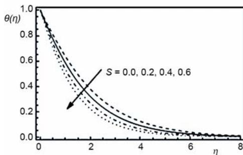
Figure 4. Temperature profiles for various values of  $S$  (suction)
