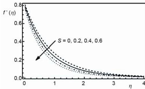
Figure 2. Velocity profiles for various values of  $S$  (suction)
