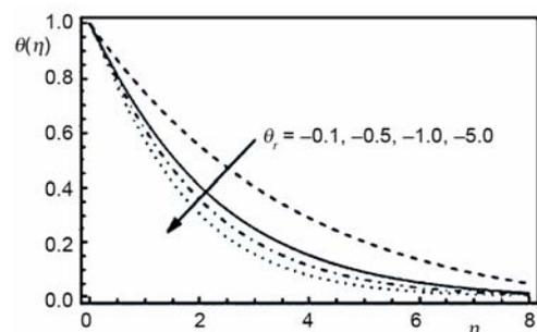
Figure 11. Temperature profiles for various values of  $\theta_r$
