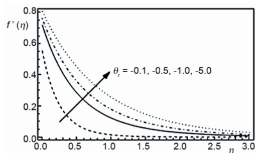
Figure 10. Velocity profiles for various values of  $\theta_r$
