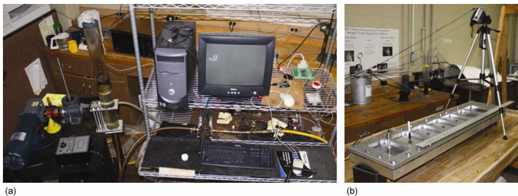
Figure 2. The 1-D flow experiment set-up, (a) data acquisition system, (b) the 1-D mold set-up (for color image see journal web-site)
