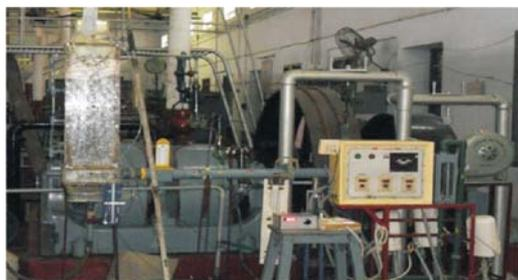
Figure 1(a). Snap shot of the experimental set-up of forced draft cooling tower
