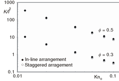
Figure 10. Logarithmic plot showing the dependence of the ratio of intrinsic permeability to distance of the mean-free path ( K/l^2 ) on the Knudsen number
