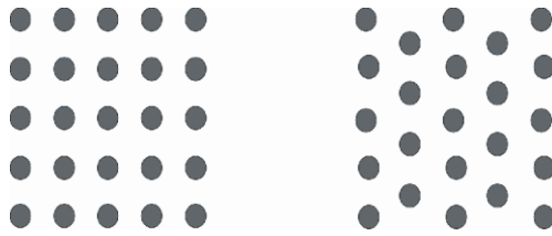
Figure 2. 2-D porous space with in-line (l. h. s.) and staggered (r. h. s.) arrangements
