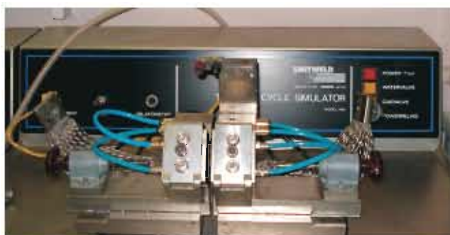
Figure 1. Heat affected zone simulator SMITWELD
