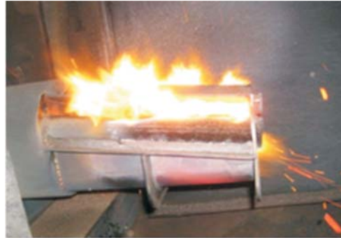
Figure 12. Combustion with optimised air supply
