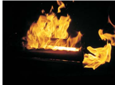
Figure 6. Combustion of wood pellets in the burner of original design
