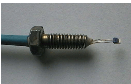
a) Adapted sensor screw for measuring temperatures of the gas in the pipe
