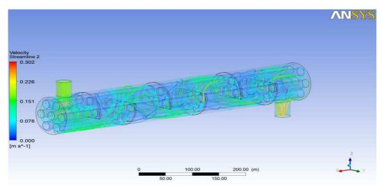
Figure 3. Variation of streamlines along the shell for 0° baffle inclination angle
