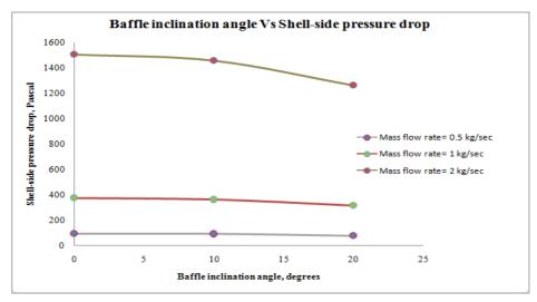
Figure 7. Variation of pressure drop with baffle inclination angle (for 0.5~kg/s, 1~kg/s, 2~kg/s mass flow rates)
