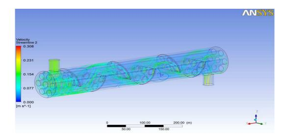
Figure 5. Variation of streamlines along the shell for 20° baffle inclination angle
