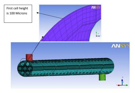
Figure 2. Discretised fluid domain with non uniform mesh for capturing boundary layer
