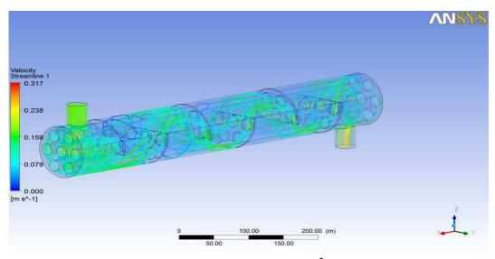
Figure 4. Variation of streamlines along the shell for 10° baffle inclination angle
