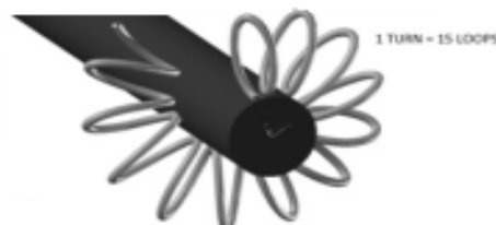
Fig.2d.Details of one turn of the Wire coiled coil matrix turbulator
