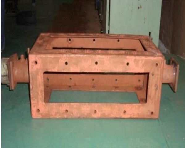
Figure 6 Cast Iron Frame
