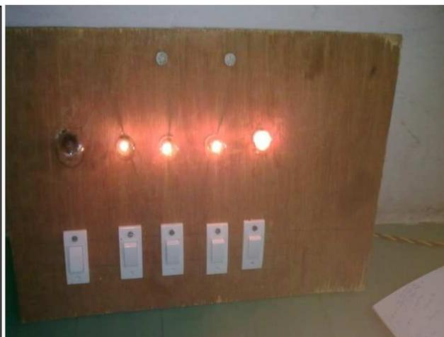
Fig. 18 Electric bulb load panel
