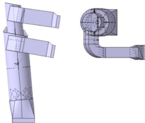
**Figure 6. Reconstruction of the aero-mixture splitter – change of the angle from  $15^\circ$  to  $5^\circ$  and reduction to circular cross-section**
