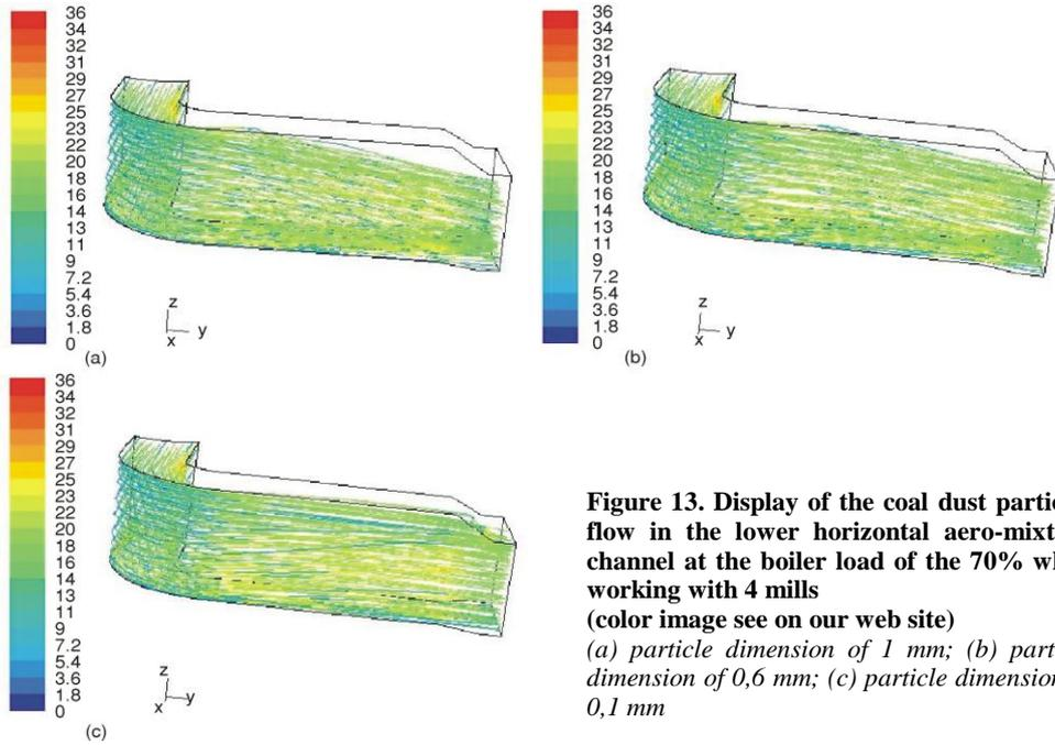
**Figure 13. Display of the coal dust particles flow in the lower horizontal aero-mixture channel at the boiler load of the 70% while working with 4 mills**
