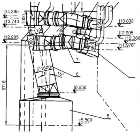
**Figure 7. Transitional piece between the separator and splitter – reduction**
