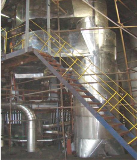
**Figure 11. Reconstructed aero-mixture splitter**
