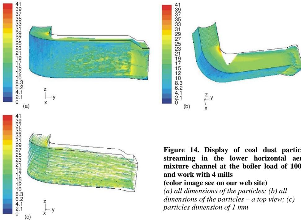
**Figure 14. Display of coal dust particles streaming in the lower horizontal aero-mixture channel at the boiler load of 100% and work with 4 mills**
