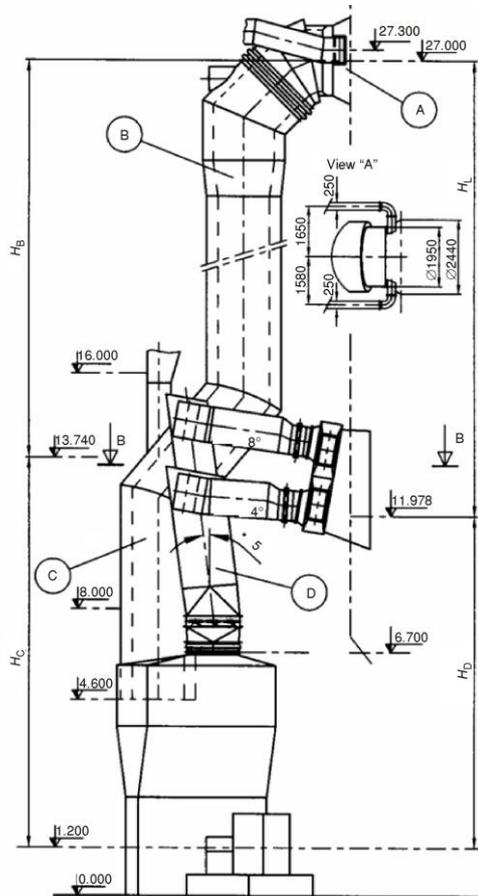
**Figure 9. Reconstructed aero-mixture channels of mill plant No. 3 with classification in the sections and elements**
