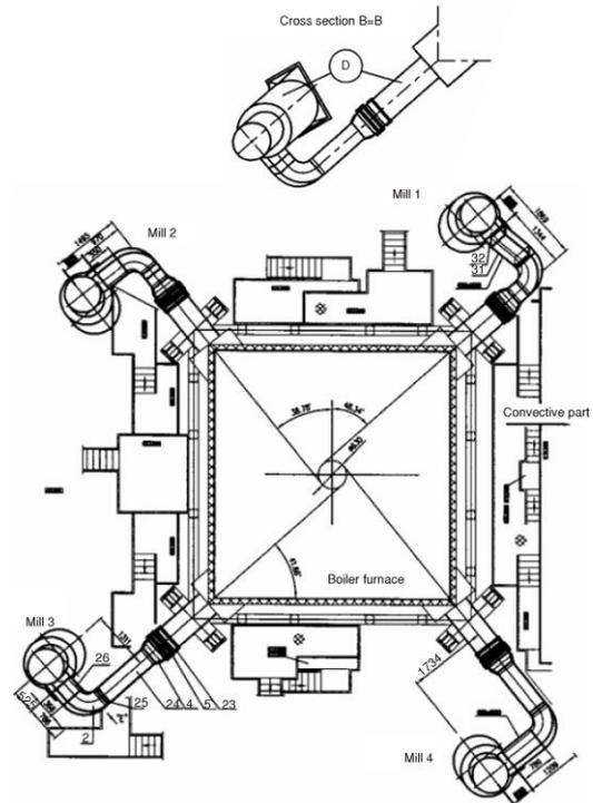
**Figure 10. The cross-section of boiler furnace and burners with belonging fan mills – recirculation channels**
