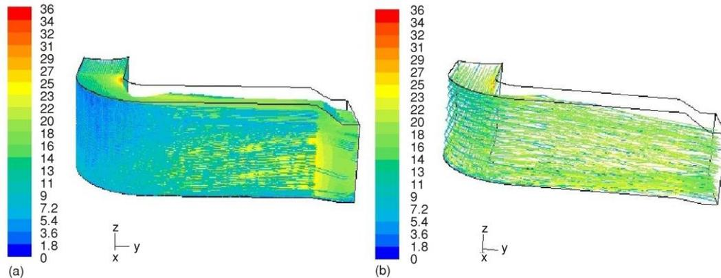
**Figure 15. Display of coal dust particles streaming in the lower horizontal aero-mixture channel at the boiler load of 85% and work with 4 mills (color image see on our web site)**
