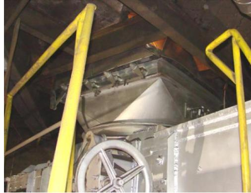
**Figure 8. Transition piece – the reduction to a circular cross-section**
