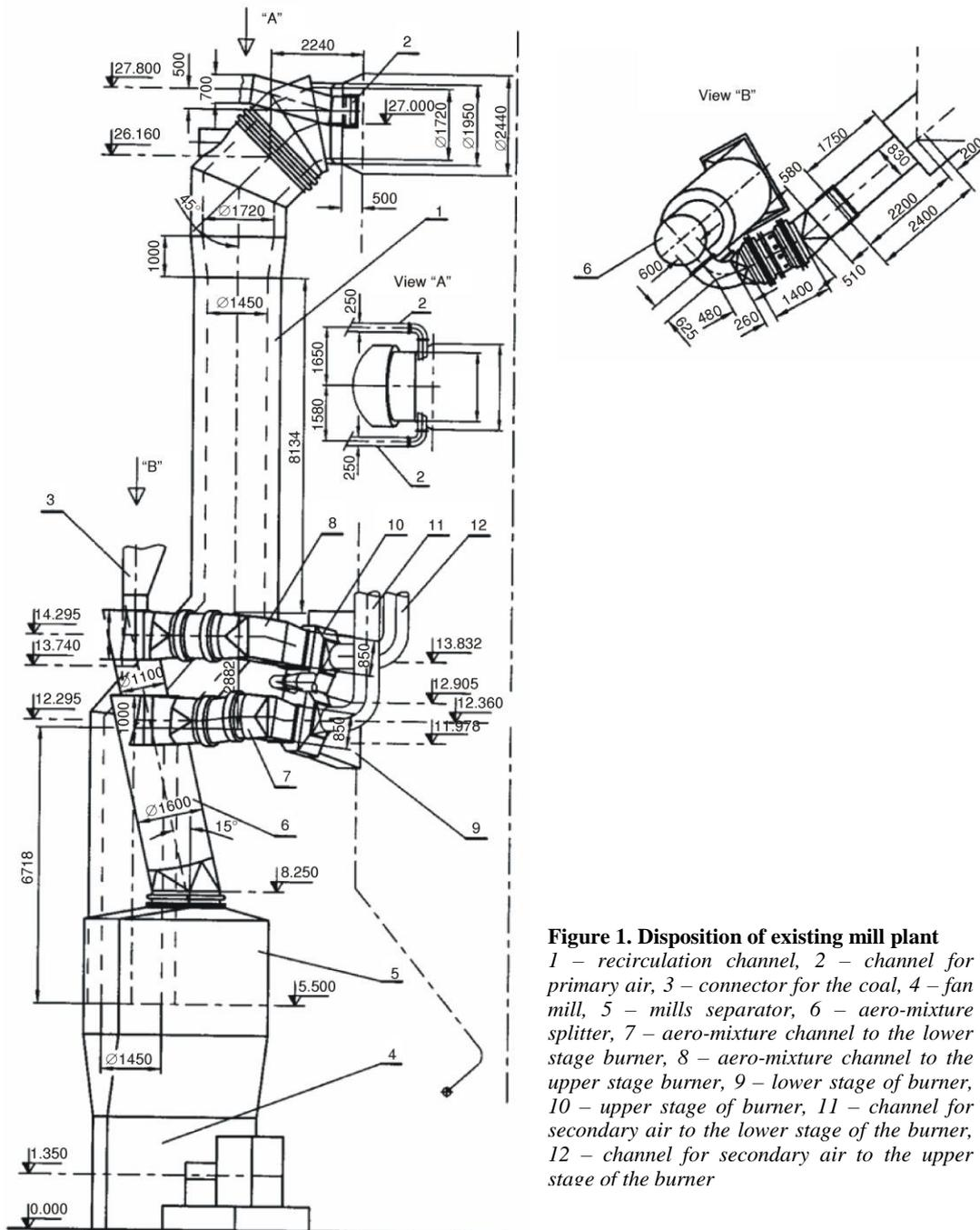
**Figure 1. Disposition of existing mill plant**
