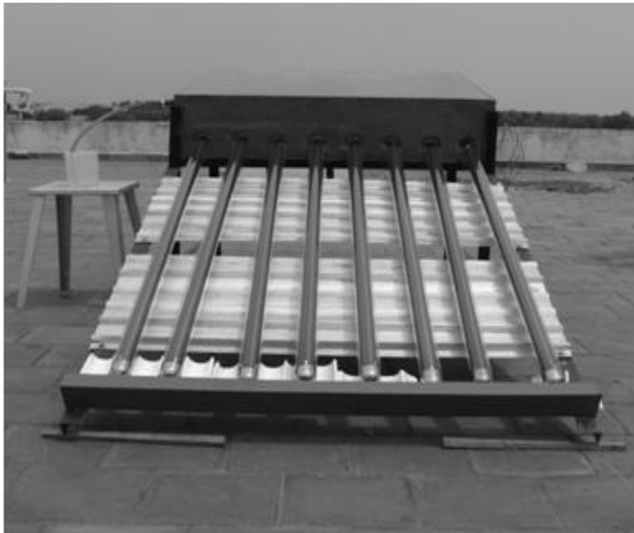
Figure 3. Pictorial view of solar still augmented with evacuated tubes
