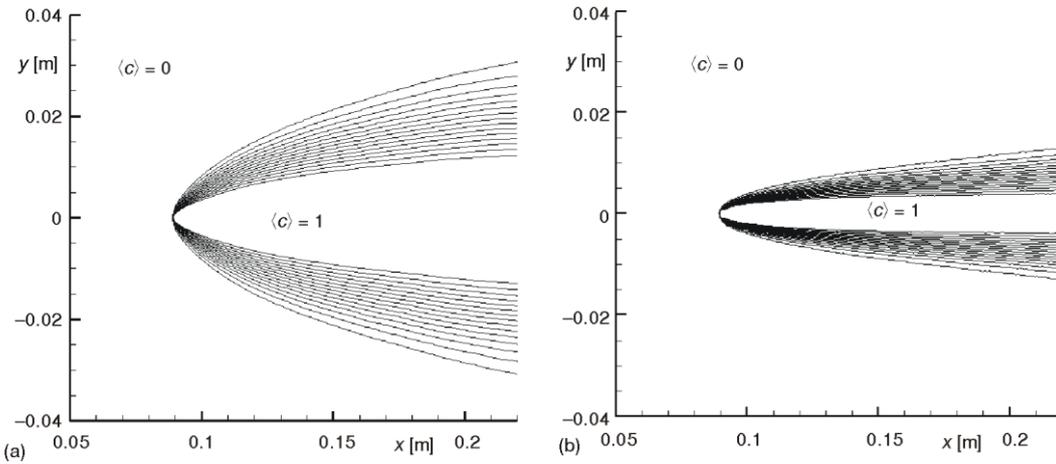
**Figure 4.** Field of mean progress variable for equivalence ratio  $\phi = 1$  and for two values of turbulence intensity, respectively,  $I = 9\%$  (a) and  $I = 4\%$  (b)
