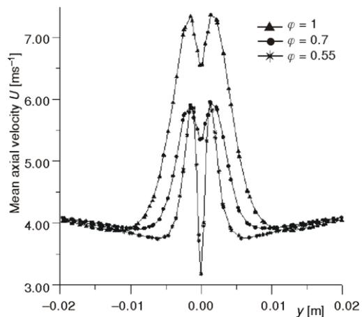
**Figure 8.** Axial distributions of mean velocity just after the wire for turbulence intensity  $I = 9\%$
