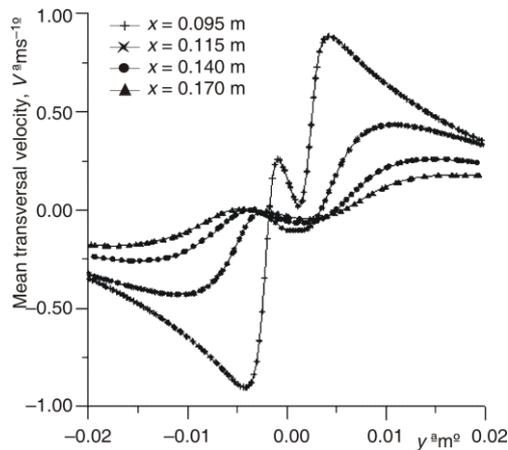
Figure 10. Transverse mean velocity for an equivalence ratio,  $\phi = 0.55$  and turbulence intensity,  $I = 9\%$
