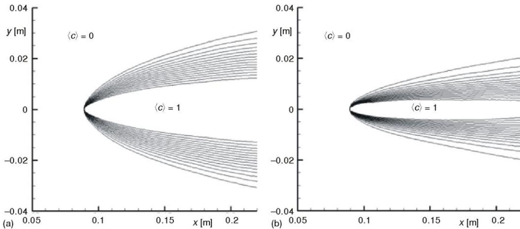
**Figure 3.** Field of mean progress variable for turbulence intensity  $I = 9\%$  and for two values of equivalence ratio, respectively,  $\phi = 1$  (a) and  $\phi = 0.55$  (b)
