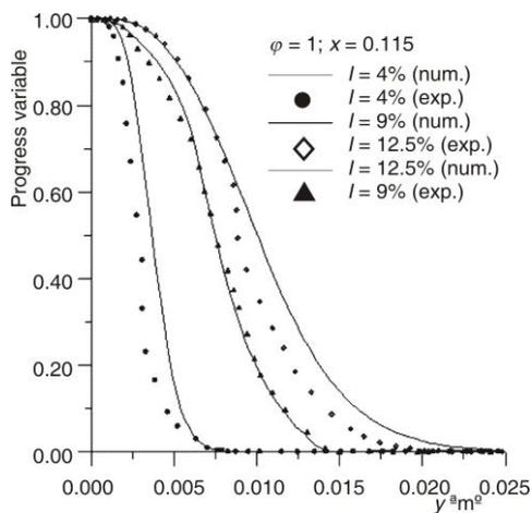
**Figure 7.** Transverse distributions of mean progress variable for equivalence ratio  $\varphi = 1$  at  $x = 0.115$  m
