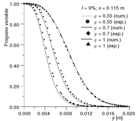
**Figure 6.** Progress variable at  $x = 0.115$  m for turbulence intensity  $I = 9\%$
