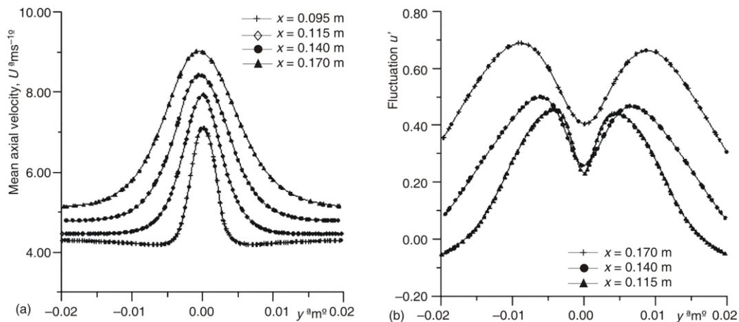
Figure 9. Profiles of the axial mean (a) and fluctuation (b) velocity for  $\phi = 0.55$  and  $I = 9\%$  turbulence
