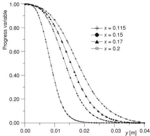
**Figure 5.** Transverse distributions of mean progress variable for equivalence ratio  $\varphi = 1$  and for turbulence intensity  $I = 9\%$
