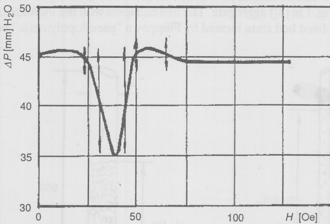
Figure 2. Pressure drop as a function of the magnetic field intensity. The arrows indicate the pressure drop pulsations. Filippov [11]; Water-magnetite, h_{b0} = 11, 2 cm. Undefined liquid velocity
