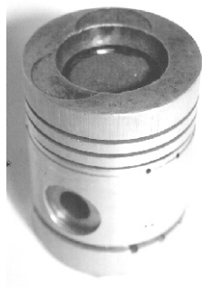
Cup head piston of diesel engine fitted with porous material disc in cup shape and piston coated with SiC
