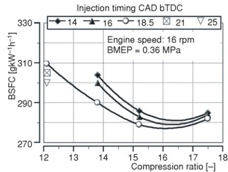
Figure 12. Effects of compression ratio and injection timing on fuel consumption
