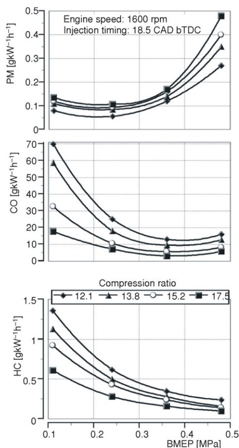
Figure 11. Effects of compression ratio and BMEP on engine exhaust emissions
