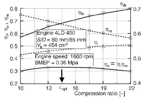
Figure 5. Influence of compression ratio on mechanical, theoretical, indicated, and brake thermal efficiency [2]
