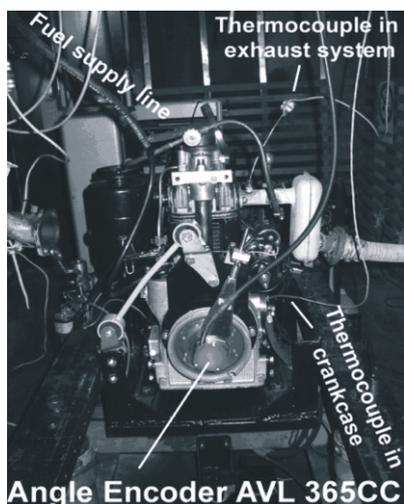
**Figure 7. The experimental engine**
