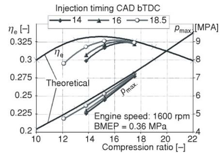
Figure 13. Effects of compression ratio and injection timing on brake thermal efficiency and maximal pressure
