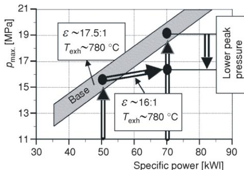
Figure 1. Specific power and maximal cylinder pressure [7]
