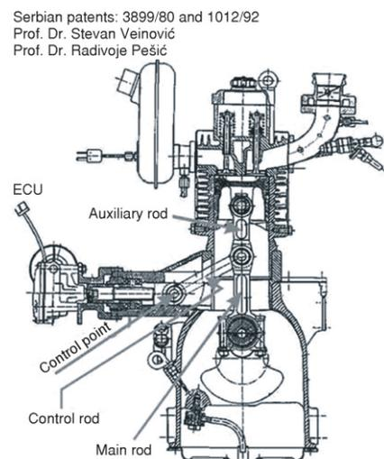
**Figure 2. Engine with automatic variable compression ratio [13, 14]**
