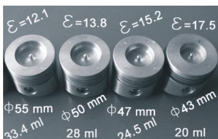
**Figure 8. Pistons before experiments**
