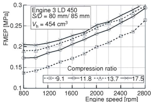
Figure 4. Compression ratio and mechanical losses – FMEP [1]
