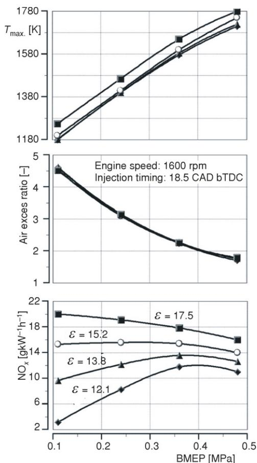
Figure 10. Effects of compression ratio and BMEP on engine performance and  $NO_x$  emission
