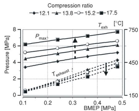
Figure 9. Effects of compression ratio and BMEP on engine performance
