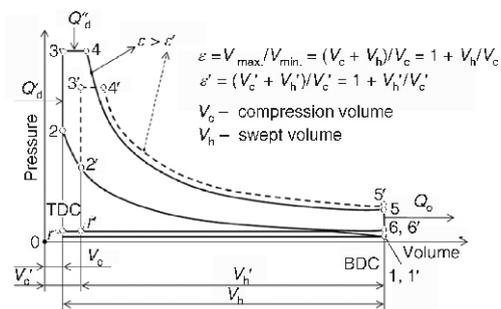
Figure 3. Comparison of ideal cycles for different values of compression ratio [1]
