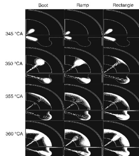
Figure 9. Plots of fuel spray, vapor, and wall impingement at three injection mode over various crank angle
