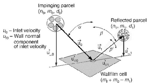
Figure 2. Wall interaction of droplets
