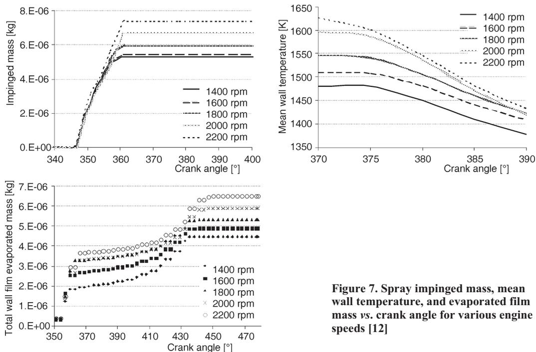
**Figure 7. Spray impinged mass, mean wall temperature, and evaporated film mass vs. crank angle for various engine speeds [12]**
