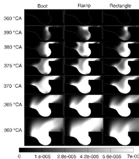
Figure 11. Plots of NO<sub>x</sub> mass fraction in cylinder at three injection mode over various crank angle
