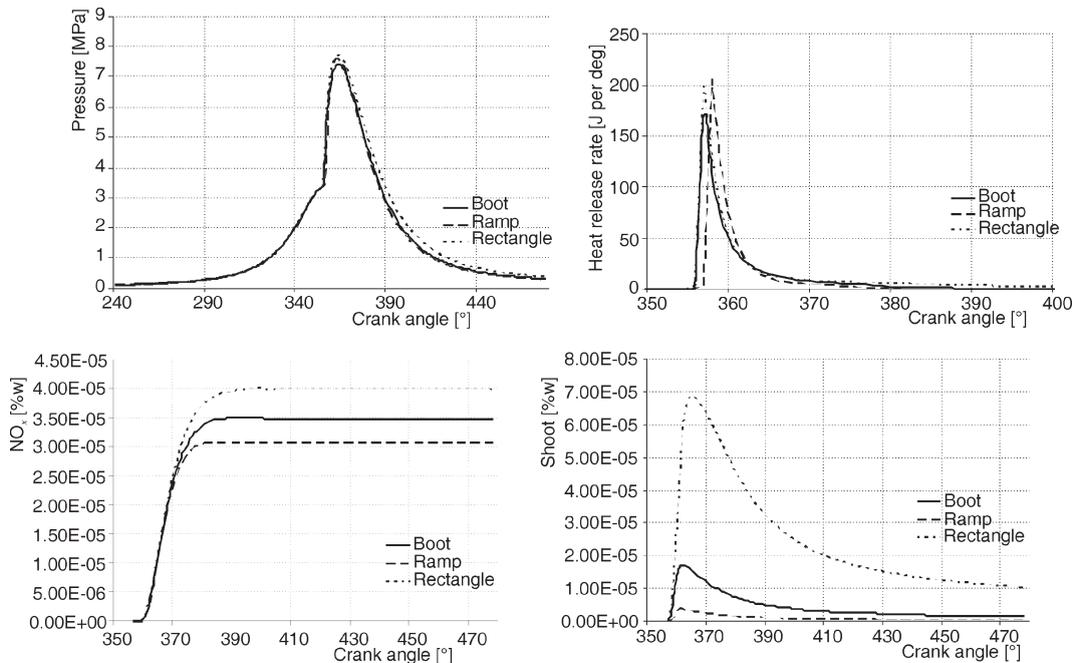
Figure 5. Mean in-cylinder pressure, heat release rate,  $\text{NO}_x$ , and soot mass fractions for different injection modes
