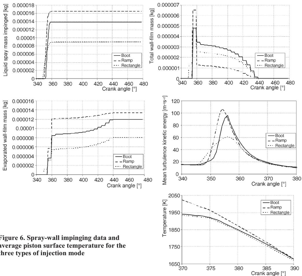
**Figure 6. Spray-wall impinging data and average piston surface temperature for the three types of injection mode**
