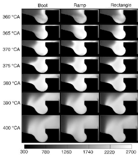
Figure 8. Plots of temperature in cylinder at three injection mode over various crank angle
