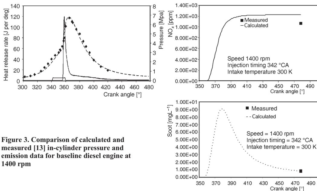
**Figure 3. Comparison of calculated and measured [13] in-cylinder pressure and emission data for baseline diesel engine at 1400 rpm**
