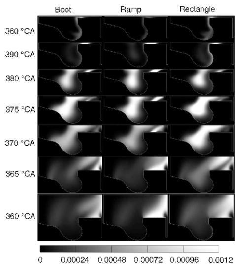
Figure 10. Plots of soot mass fraction in cylinder at three injection mode over various crank angle
