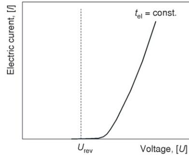
Figure 2. Example of the  $U-I$  characteristic of an electrolyzer
