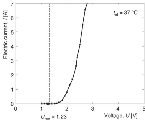
Figure 4. The reference electrolyzer  $U$ - $I$  characteristic
