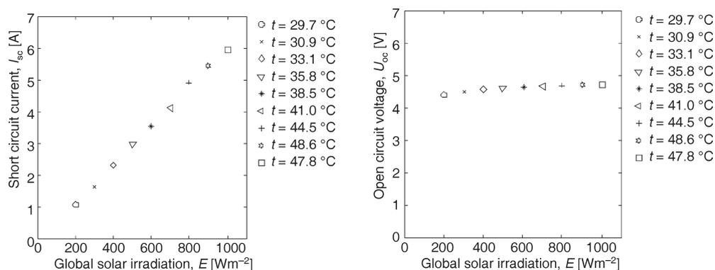
**Figure 6. Measurements of  $I_{sc}$  and  $U_{oc}$  dependence on  $E$**
