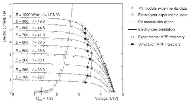
Figure 7. Comparison of mathematical models of the PV module and the electrolyzer with measurement values
