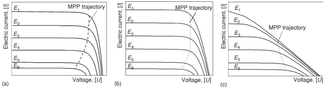
Figure 1. Examples of MPP trajectories of PV modules curving to the right, vertically, and to the left
