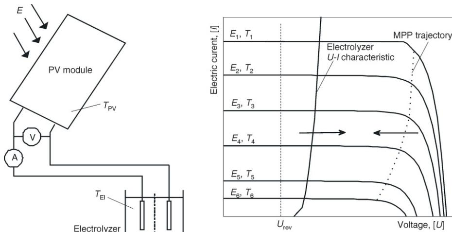
Figure 3. Example of the MPP trajectory approximately matched to the  $U-I$  characteristic
