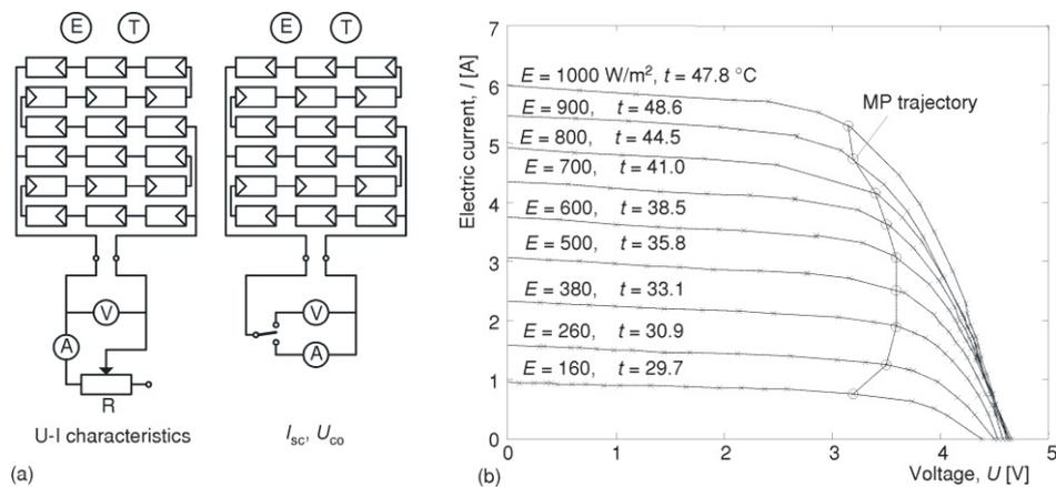
Figure 5. Diagram of the measurement process (a) and the results (b)
