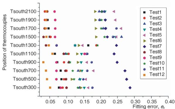
Figure 10. The minimum fitting error of fitting for TC-South
