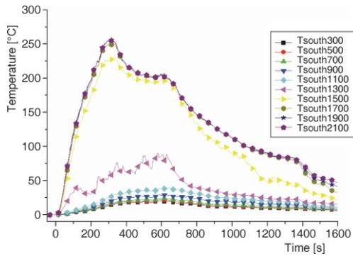
Figure 4. Compartment temperature of TC-South in Test2
