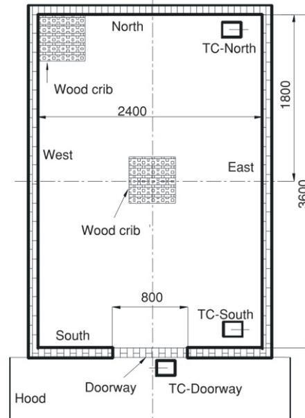
**Figure 1. Test arrangement inside ISO 9705 room**
