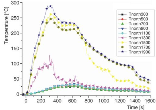
Figure 5. Compartment temperature of TC-North in Test2
