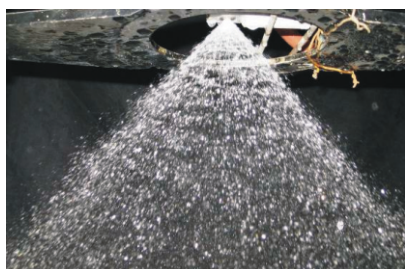
Figure 17. Fully opened spray cone under design condition ( P_f = 10 , P_0 = 4 bar)
