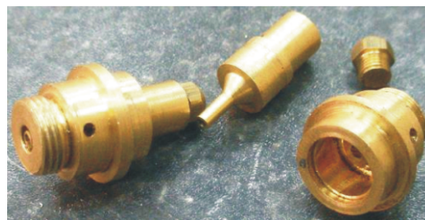
Figure 11. Assembled and disassembled of manufactured injector
