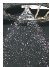
Figure 19. Spray cone angle of external nozzle
