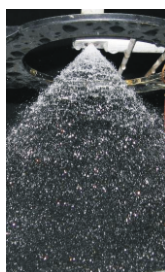
Figure 18. Spray cone angle of internal nozzle
