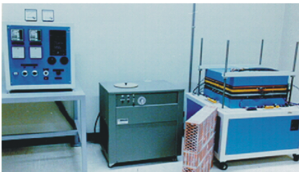
Figure 2. Guarded hotplate thermal conductivity measuring equipment
