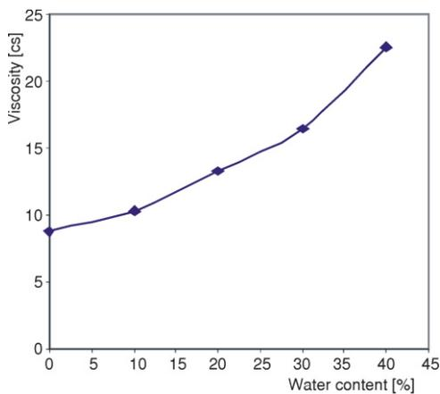
Figure 2. Viscosity at 40 °C with varying water content
