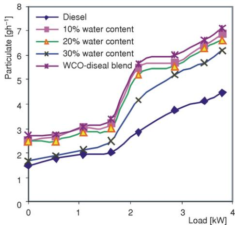
Figure 7. Variation of particulate matter with load
