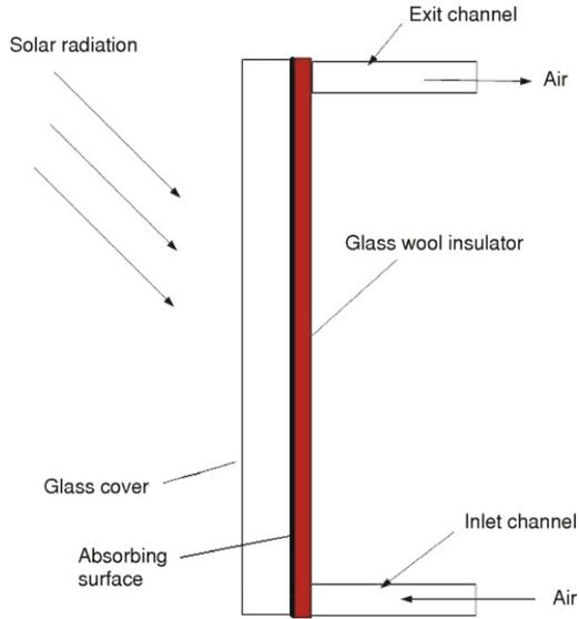
Figure 1. A schematic of the designed collector [23]
