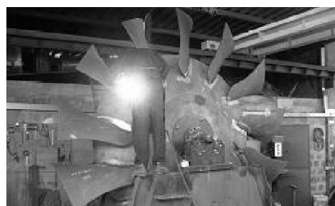
Figure 3. Ventilator production – welding of blades
