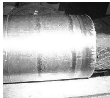
Figure 2. Damaged journal surface caused by fretting
