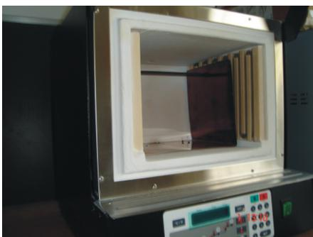
**Figure 2. Placing the radiant panels inside the working area of the furnace**
