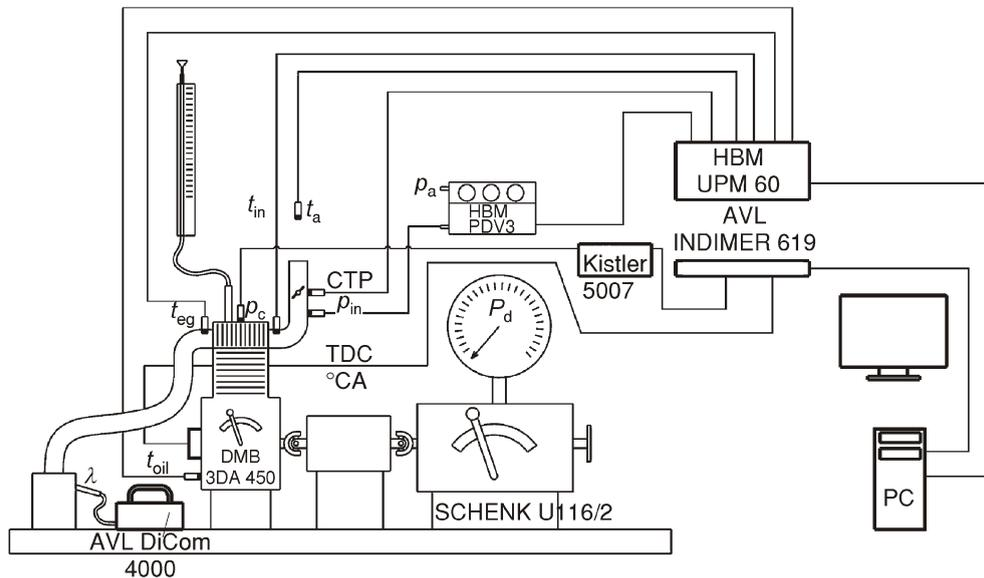
**Figure 2. Test bench and instrumentation disposition**
