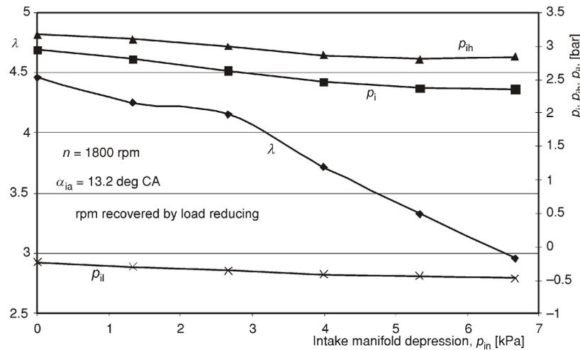
Figure 7. Intake manifold depression influence on air-fuel ratio and  $p_i$ ,  $p_{ih}$ , and  $p_{ii}$  (color image see on our web site)
