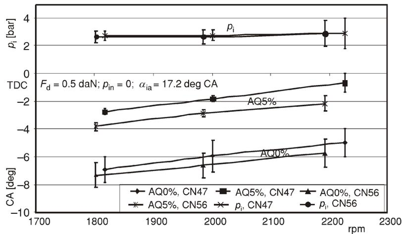
Figure 4. Influence of rpm on fuel combustion parameters for factory injection advance setting (color image see on our web site)
