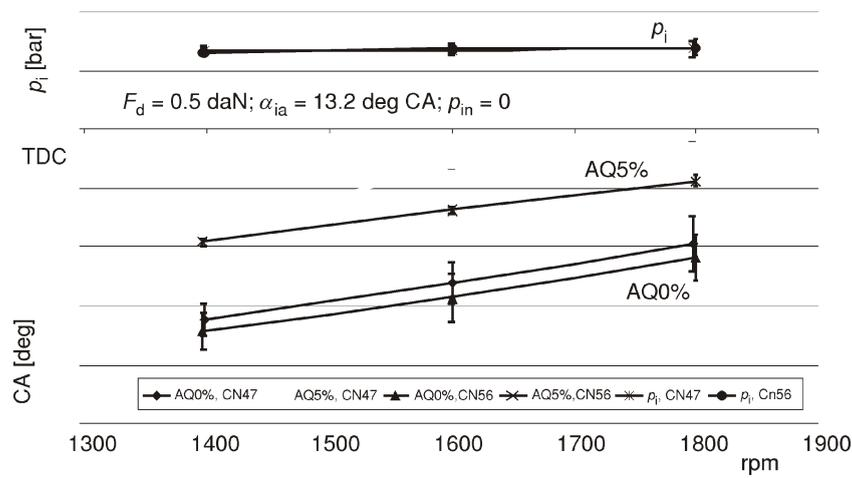
**Figure 5. Influence of rpm on fuel combustion parameters for retarded injection advance setting (color image see on our web site)**
