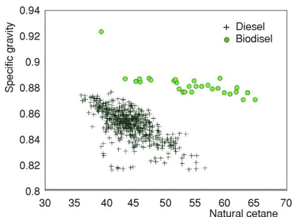
**Figure 1. Natural cetane and specific gravity of biodiesel and conventional diesel**
