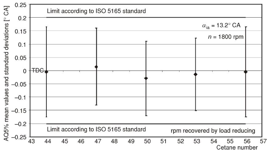
Figure 9. Start of combustion criteria precision at referent regimes (color image see on our web site)
