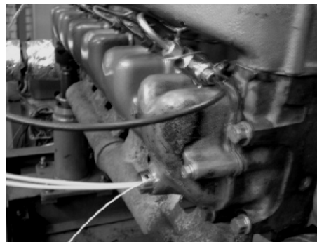
Figure 2. Location of piezoelectric sensor for pressure registration in HP line before injector
