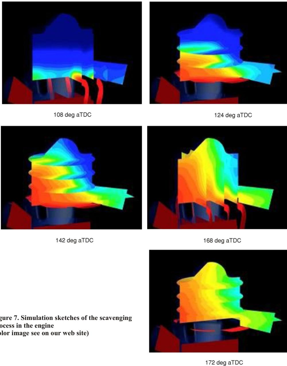
**Figure 7. Simulation sketches of the scavenging process in the engine (color image see on our web site)**
