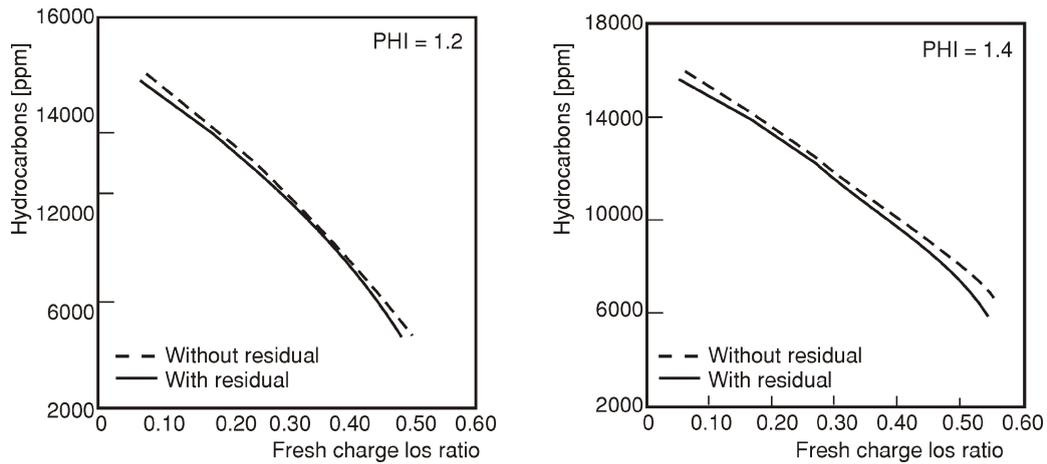
Figure 8. Effect of fresh charge loss ratio on HC concentration at different equivalence ratio (PHI  $\Phi$ )
