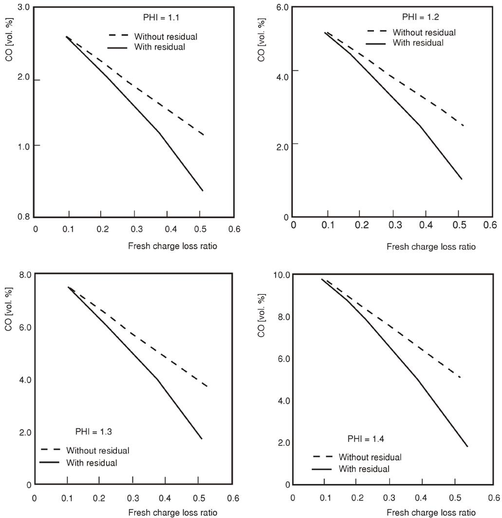
Figure 9. Effect of fresh charge loss ratio on CO concentration at different equivalence ratio (PHI  $\Phi$ )
