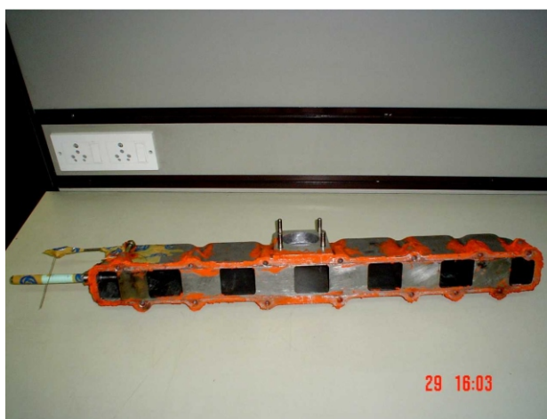
Figure 1. Experimental swirl plate set up for 2-valve port variable swirl mechanism (color image see on our web site)
