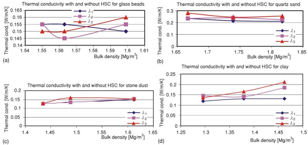
Figure 1. Thermal Conductivity with and without HSC at different packing densities
