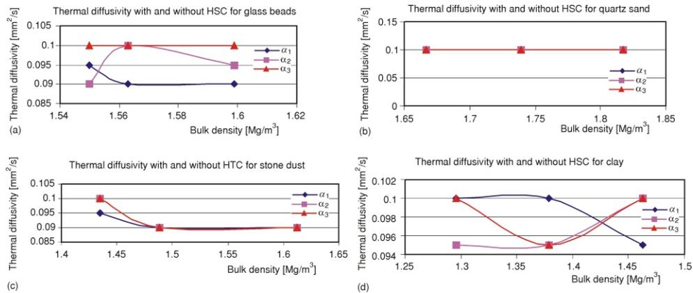
Figure 2. Thermal Diffusivities with and without HSC at different packing densities
