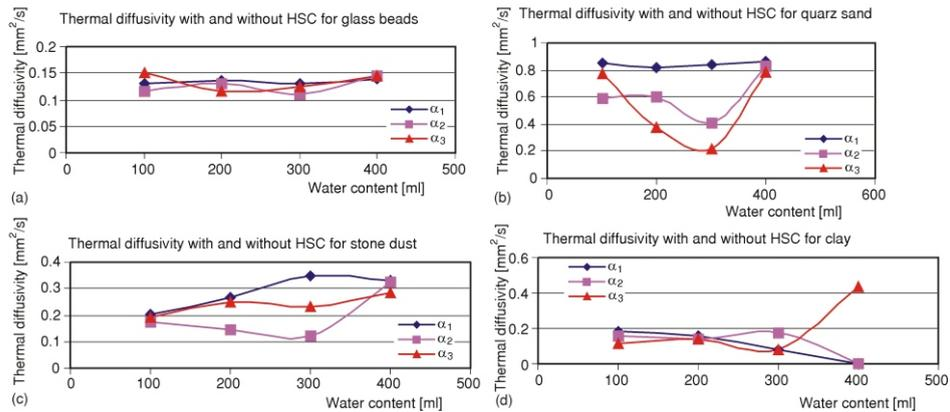
Figure 4. Thermal diffusivity with and without HSC at different water contents
