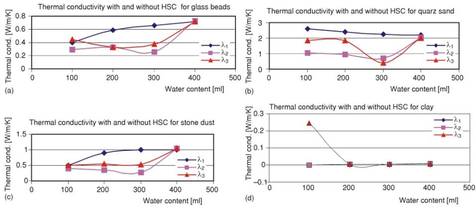
Figure 3. Thermal conductivity with and without HSC at different water contents
