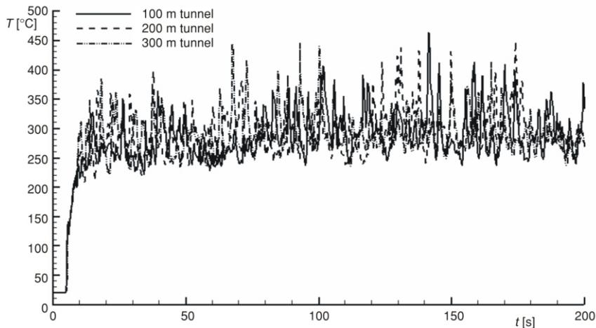
Figure 3. Comparison of thermocouple temperatures for the tunnels with different length
