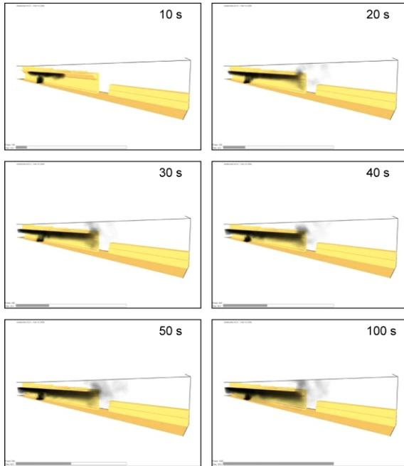
**Figure 10.** Results for the simulation with an external wind of 10 m/s (perpendicular to the tunnel axis)
