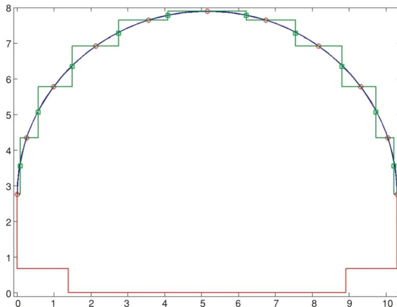
**Figure 1. Stepped approximation of the cross-section of the tunnel**
