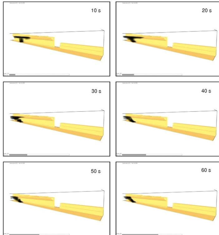
**Figure 9. Results for the simulation with an external wind of 10 m/s (parallel with the tunnel axis)**
