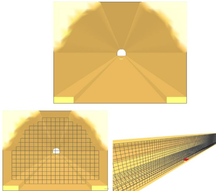
**Figure 2. Tunnel geometry in FDS and computational grid**
