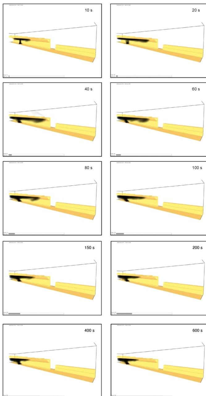
**Figure 8. Results for the simulation with an external wind of 5 m/s (parallel with the tunnel axis)**
