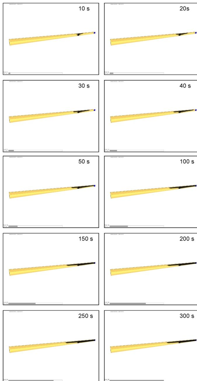
**Figure 12.** Simulation result for a 14 MW fire with a ventilation velocity of 2 m/s
