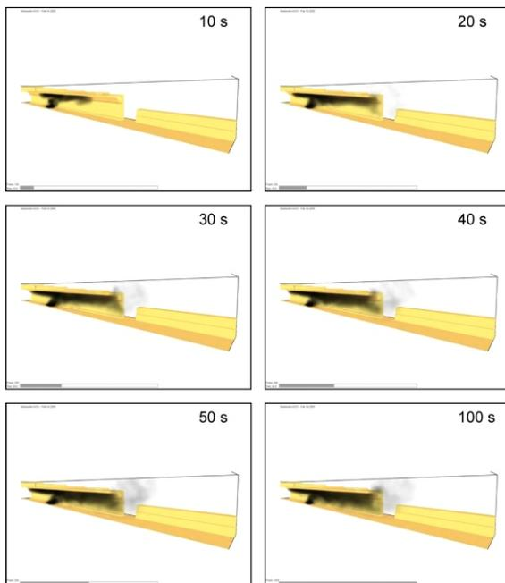
**Figure 11.** Results for the simulation with an external wind of 20 m/s (perpendicular to the tunnel axis)
