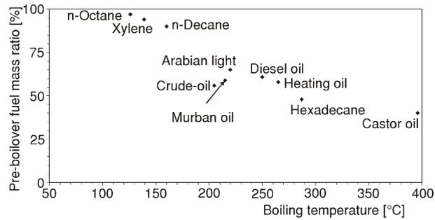
**Figure 6. Pre-boilover fuel mass ratio plotted as a function of boiling point for the various fuels (operating conditions: pure fuels – pan diameter 15 cm, multi-component fuels – pan diameter 30 cm)**
