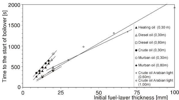
**Figure 3. Time to the start of boilover as a function of initial fuel-layer thickness for the multicomponent fuels (pan diameter is bracketed)**
