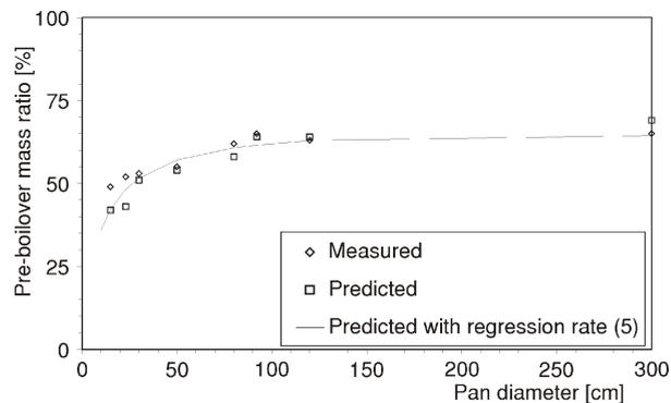
**Figure 15. Comparison between measured and predicted pre-boilover fuel mass ratio plotted as a function of pan diameter (fuel: heating-oil – initial fuel-layer thickness 13 mm)**
