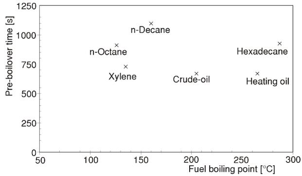
**Figure 5. Pre-boilover time as a function of fuel boiling point (initial fuel-layer thickness: 13 mm, pan diameter: 15 cm)**
