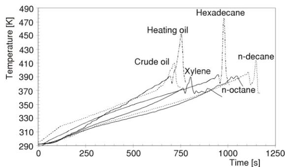
**Figure 12. Fuel/water interface temperature as a function of time (initial fuel-layer thickness: 13 mm, pan diameter: 15 cm)**
