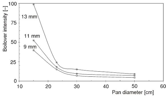
**Figure 7. Boilover intensity as a function of the initial fuel-layer thickness for different pan diameters and initial fuel-layer thicknesses (fuel: crude-oil, initial fuel-layer thickness is bracketed)**
