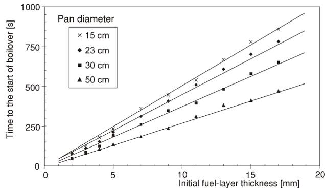
If the regression rate of the fuel surface is known, then it is possible to deduce, by difference from the fitted slope, the effective thermal penetration rate responsible for boilover.
