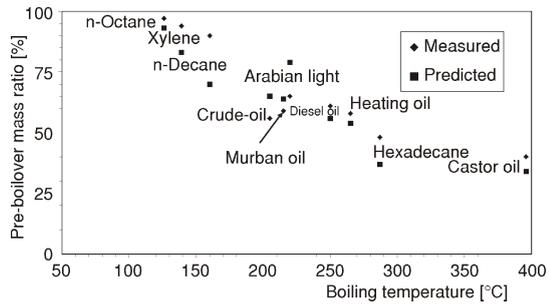
**Figure 14. Comparison between measured and predicted pre-boilover fuel mass ratio plotted as a function of boiling point for the various fuels (operating conditions: pure fuels – pan diameter 15 cm, multicomponent fuels – pan diameter 30 cm)**
