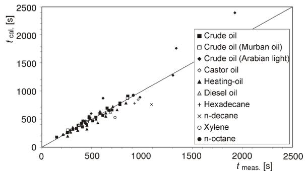
The prediction of the analysis agrees satisfactorily ( $\leq 20\%$ ), as well for the results obtained at small-scale as for those obtained with the larger pool sizes (1 or 3 m in diameter). Some calculated values are in excellent agreement with measurements, other show discrepancies (only two measurements – fuel: Arabian light, conditions: initial fuel-layer thickness 35 mm and pan diameter 30 cm; initial fuel-layer thickness 69 mm
