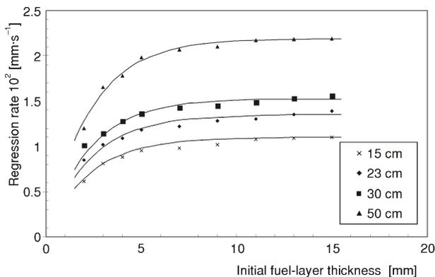
**Figure 1. Surface regression rate as a function of fuel-layer thickness for different pool diameters (fuel: crude-oil)**
