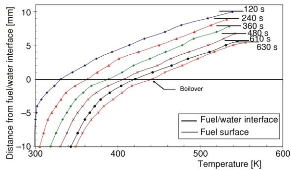
**Figure 10. Development of vertical temperature profile (pan of 15 cm in diameter and initial heating-oil thickness of 11 mm)**
