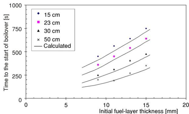
**Figure 17. Measured and calculated time to the start of boilover as a function of initial fuel-layer thickness and for different pan diameters, for heating oil**
