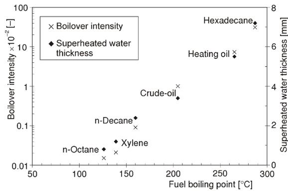
**Figure 8. Boilover intensity and superheated water thickness as a function of the difference between fuel and water boiling point (initial fuel-layer thickness: 13 mm, pan diameter: 15 cm)**
