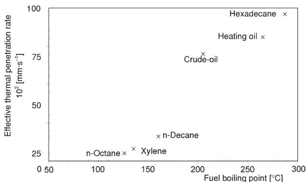
**Figure 4. Effective thermal penetration rate as a function of fuel boiling point (initial fuel-layer thickness: 13 mm, pan diameter: 15 cm)**
