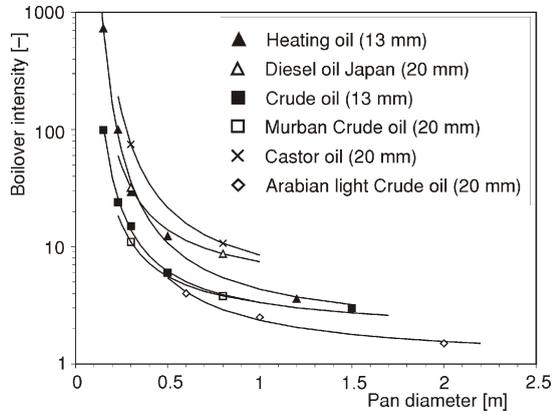
**Figure 9. Boilover intensity as a function of pan diameter (multicomponent fuels; initial fuel-layer thickness is backeted)**
