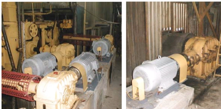
Figure 10. Drive motors of the new drive
