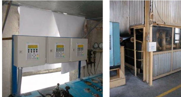
Figure 12. Control panels for press drives (left side) and one drying group (right side)
