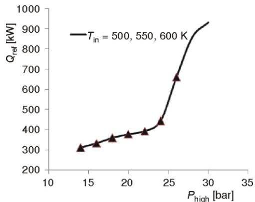
Figure 6. Effect of turbine inlet pressure on refrigeration output for different heat source temperature
