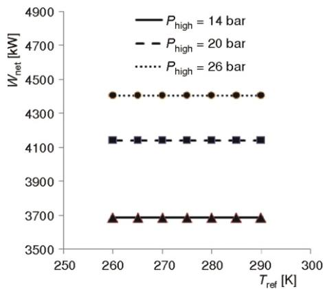
**Figure 8. Effect of refrigeration temperature on net power output for different turbine inlet pressures**
