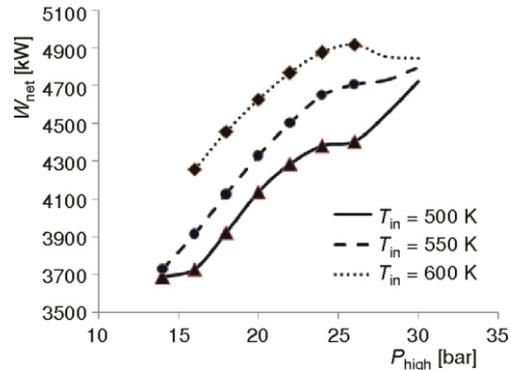
Figure 5. Effect of turbine inlet pressure on net power output for different heat source temperature
