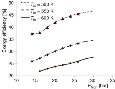
**Figure 7. Effect of turbine inlet pressure on exergy efficiency for different heat source temperature**
