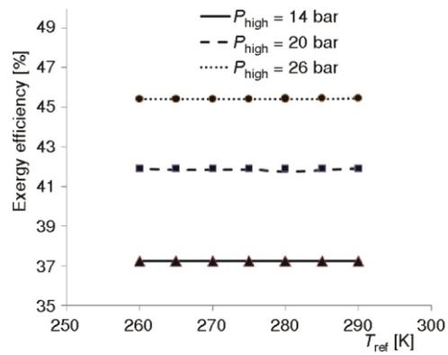
**Figure 10.** Effect of refrigeration temperature on exergy efficiency for different turbine inlet pressures
