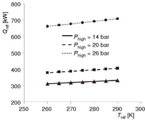
**Figure 9.** Effect of refrigeration temperature on cooling capacity for different turbine inlet pressures
