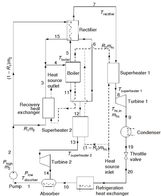
Figure 1. Schematic diagram of the combined power and refrigeration cycle
