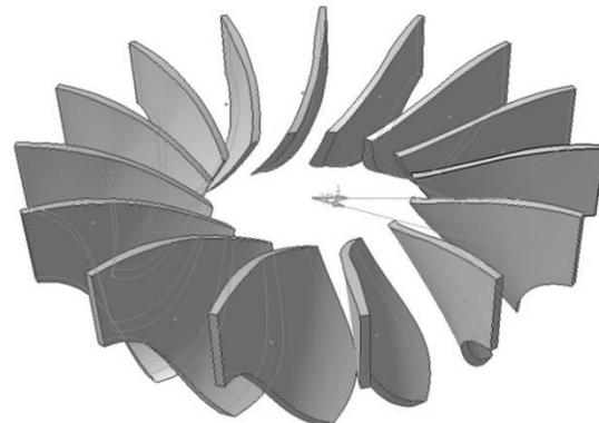
**Figure 9.** Impeller with 15 blades formed using command “Circular pattern”
