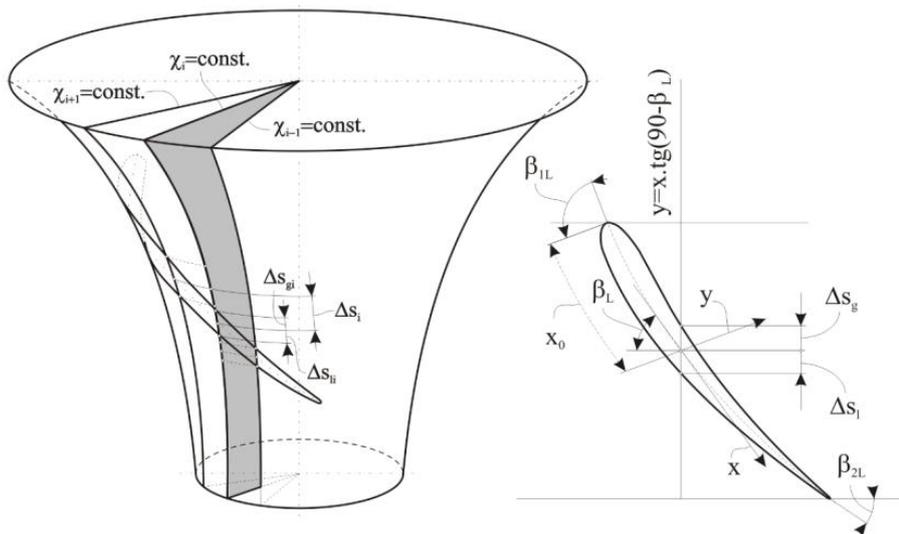
**Figure 1. Random axisymmetric stream surface of Francis turbine impeller (left) and penetration of a blade through axisymmetric stream surface (right)**
