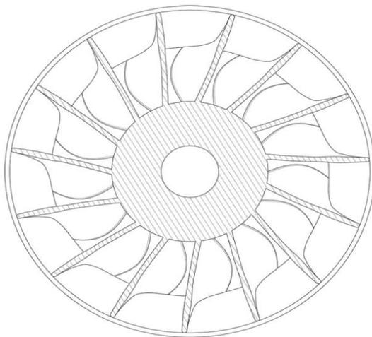
**Figure 13. Example of the sections of the impeller suitable for molding**
