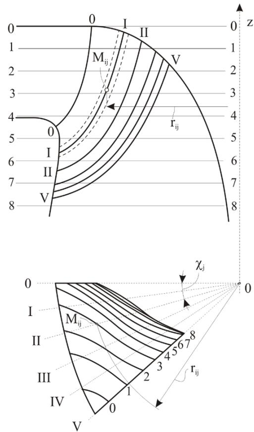
Figure 5. Cross section of the blades in meridional and circular plane suitable for molding
