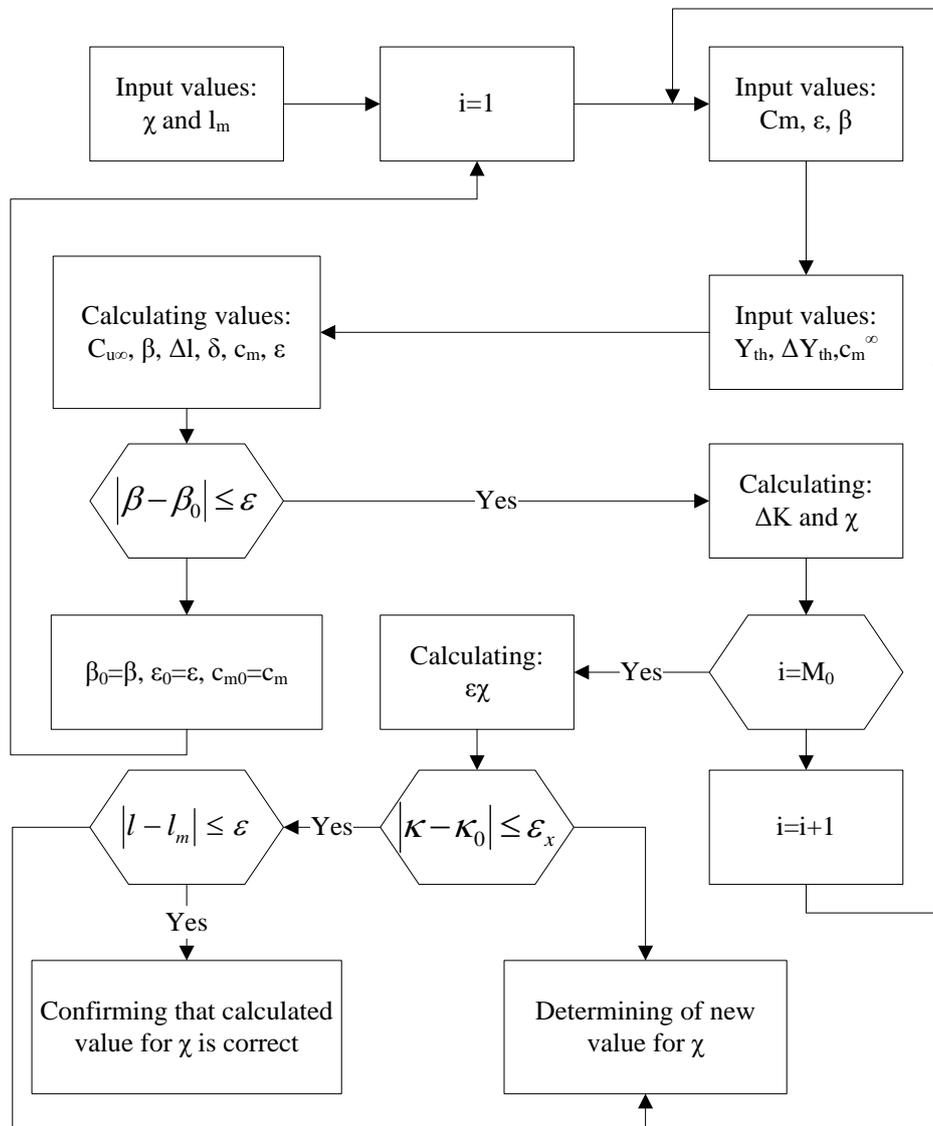
Figure 3. Algorithm for calculating blade angle in circular plane of the impeller
