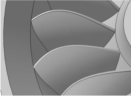
**Figure 11. Using command “Tritangent fillet” (marked surface) for final shaping of impeller’s blades entrance, exit and interblade space**
