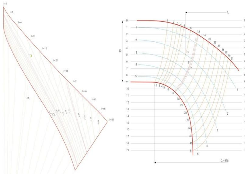
**Figure 6.** Cross section of the blades in meridional and circular plane suitable for molding retrieved from original methodology. Together with additional coordinates these cross sections represent starting points for impeller 3-D model development (circular projection – left, meridional projection – right).
