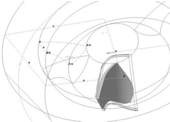
**Figure 8.** Defining profiles for “cutting” and forming entrance and exit blade curve
