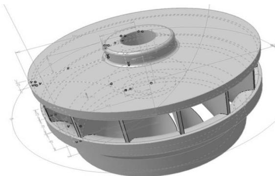
**Figure 10.** Adding impeller’s “body”
