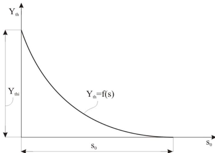
**Figure 2. The most eligible curve shape of the available energy for energy transfer in the impeller axisymmetric segments**
