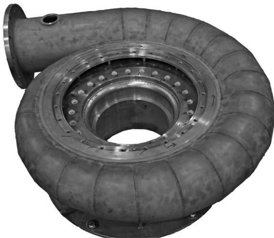
**Figure 18.** Photography of produced volute casing of SHPP turbine "Bosna 1"
