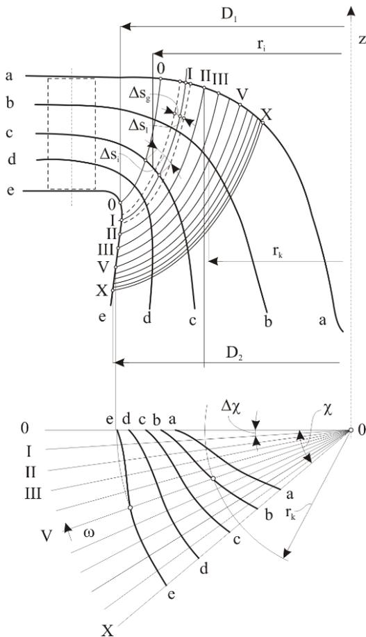
Figure 4. Impeller axisymmetric segments of small turbine (top) and radial cross section of the blades in meridional and circular plane (bottom)
