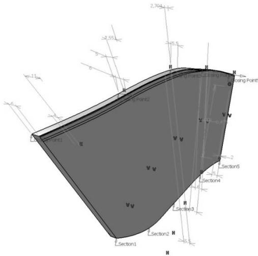
**Figure 7.** Impeller blade of SHPP turbine “Bosna 1” defined by calculated values
