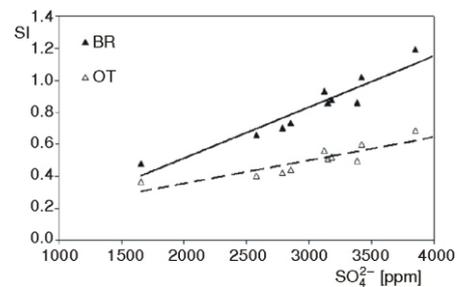
**Figure 4.** The effect of sulfate ion concentration in the feed for different feed water composition in different intakes from the Arabian Gulf
