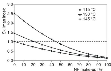
**Figure 6. Influence of NF on sulfate scale potential in BR-MSF plant**
