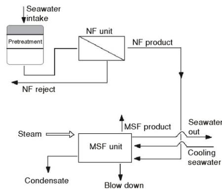
Figure 5. Schematic flow diagram of di-hybrid NF-MSF desalination system [20]
