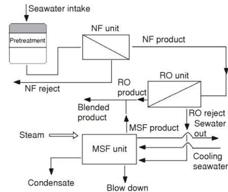
**Figure 9. Schematic flow diagram of tri-hybrid NF-RO-MSF desalination system [20]**
