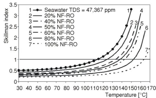
**Figure 10. Scale potential in tri-hybrid NF-RO-MSF plant at RO recovery of 60%**
