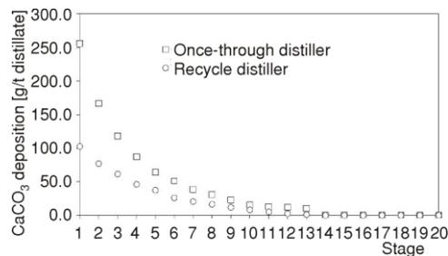
**Figure 3.** The  $\text{CaCO}_3$  deposition rates in the individual stages flash chambers of the MSF once-through and recycle distillers
