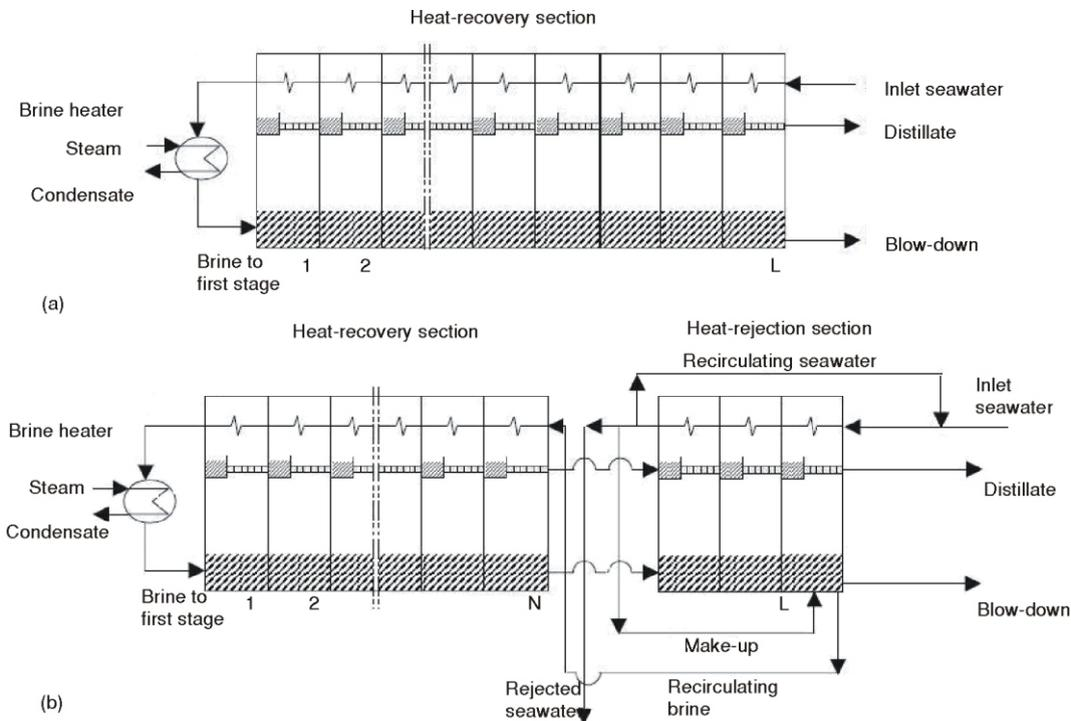
Figure 1. MSF process: (a) once-through distiller and (b) recycle distillers [12]
