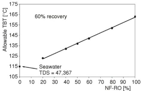
**Figure 11. Influence of NF on the allowable TBT in tri-hybrid NF-RO-MSF plant**
