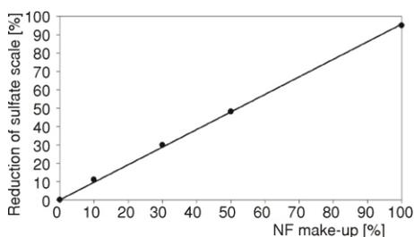
**Figure 8. Influence of NF on sulfate scale in MSF-BR plant**
