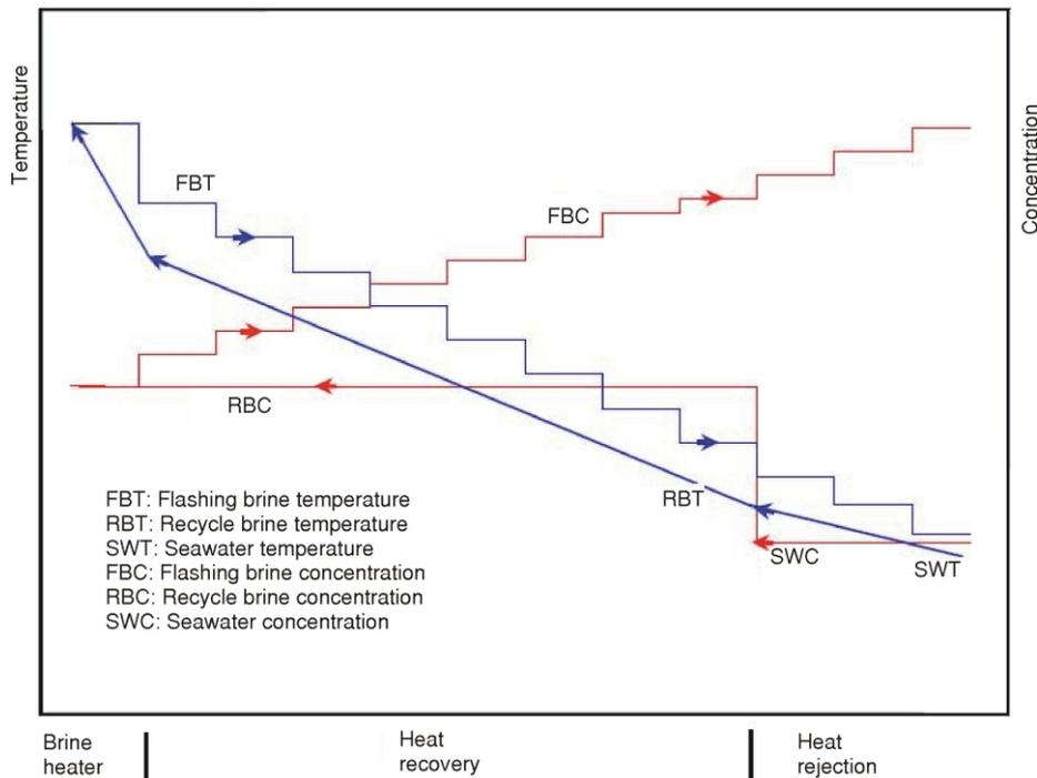
Figure 2. Temperature and concentration gradients in MSF distillers
