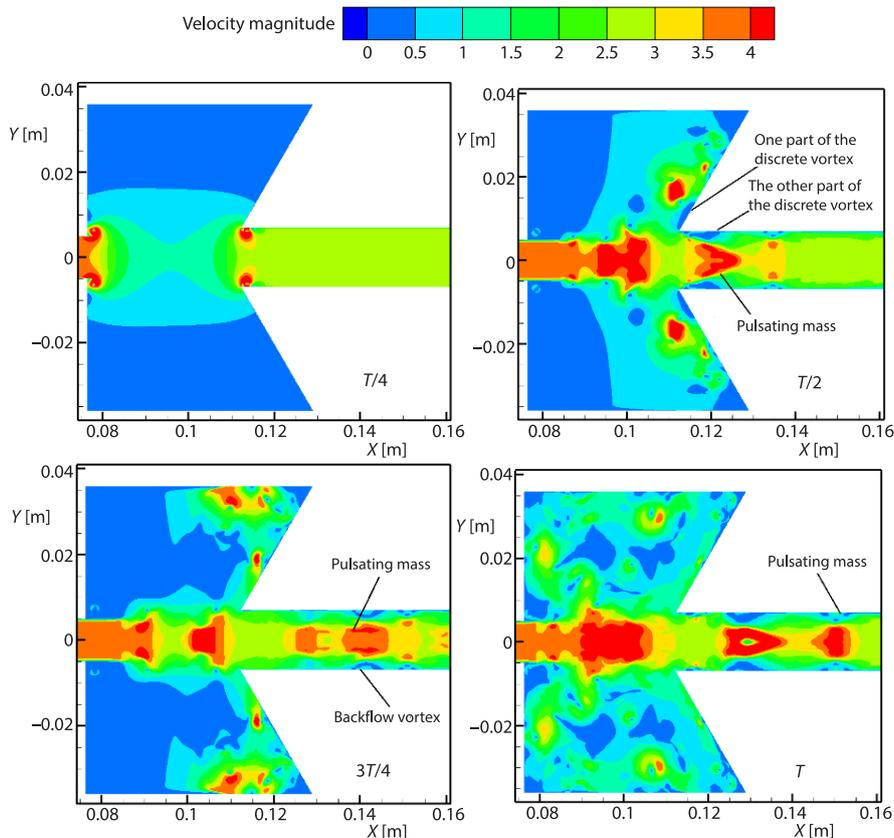
**Figure 5. Cloud diagram of velocity in self-excited oscillation chamber in one cycle**
