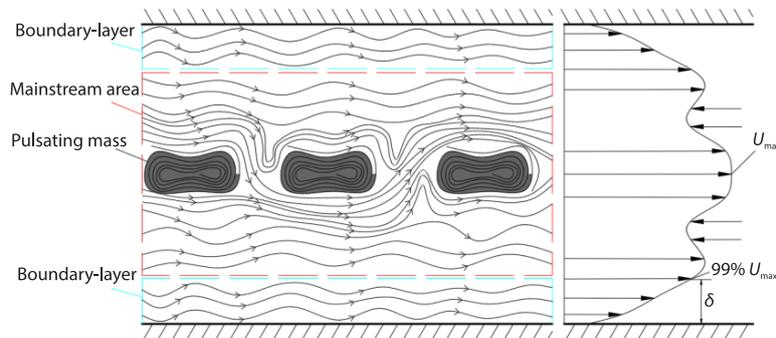
Figure 1. Disturbance effect of pulsating flow in self-excited oscillation hot runner
