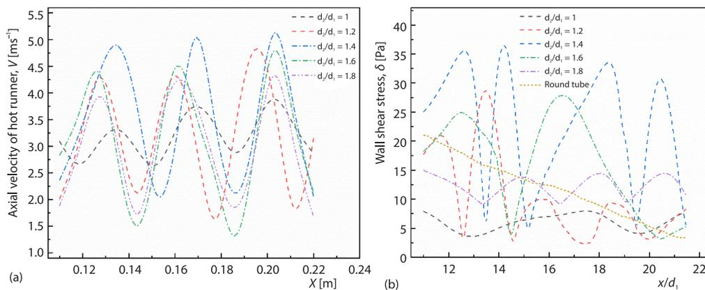
**Figure 7. Velocity at the axis center of the hot runner (a) and wall shear stress (b) under different upstream and downstream pipe diameter ratios**
