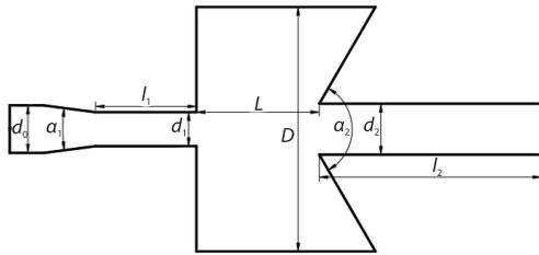
Figure 3. Structure of self-excited oscillation chamber
