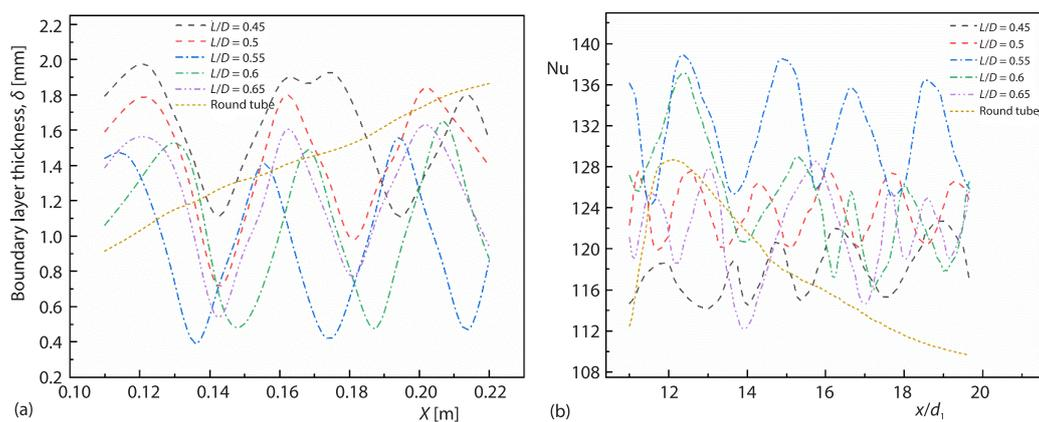
Figure 8. Boundary-layer thickness of hot runner (a) and Nusselt number curve of wall (b) under different cavity diameter ratio
