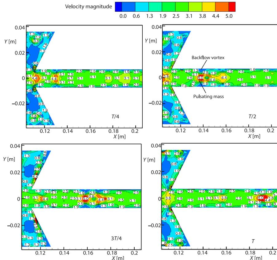
Figure 6. The evolution of pulsating flow in the self-excited oscillating hot runner
