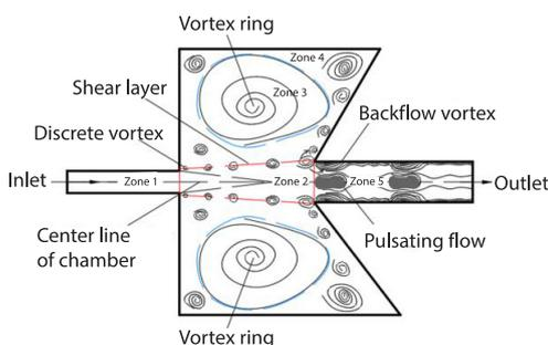
Figure 2. Schematic diagram of the formation of pulsating flow in self-excited oscillation
