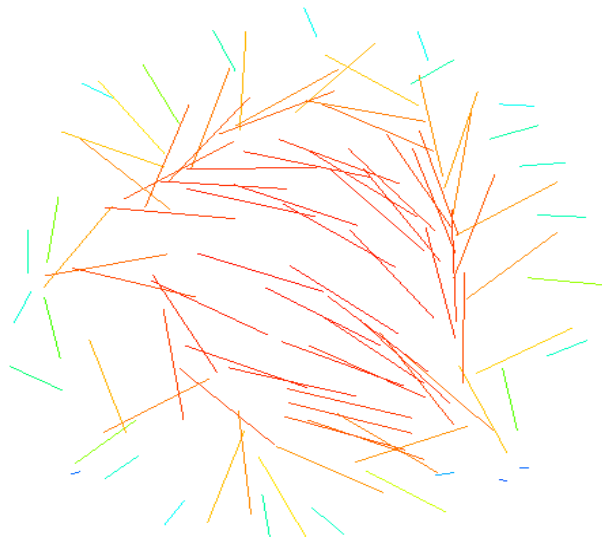
Figure 10. The view of velocity vectors in the r-q plane in a wavy tube heat exchanger.
